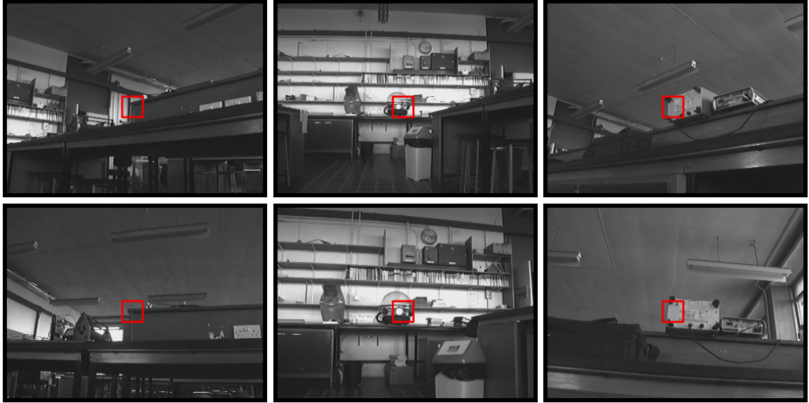
Figure 4.3: Features matched with normalised sum-of-squared-difference correlation showing the wide changes in viewing distance and direction which can be accommodated.
