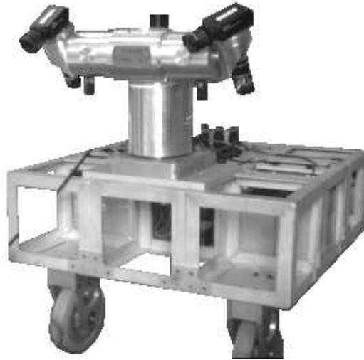
Figure 2.1: The robot used in this thesis comprises an active binocular head, equipped with two video cameras, mounted on a three-wheeled vehicle.
