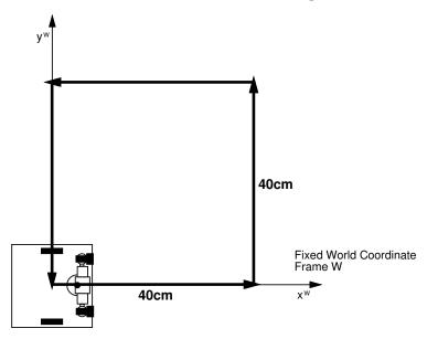
We have tape measures and scissors to borrow, and a big roll of stiff paper. Using a pen, on your paper measure and mark out an accurate square course of side length 40cm for the robot to follow, starting at one corner, defining a coordinate frame as shown above.
