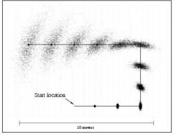
Your key aim this week is to write a program which represents the uncertain motion of your moving robot in a similar way via a particle distribution, and displays the results in the form of a cloud of particles drawn in real-time using our Pi web interface (see below).
