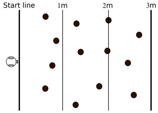
The robot will start behind a start line marked on the floor, facing forwards, and there will be a parallel goal line 3m ahead. We will mark intermediate lines at 1m and 2m. The course will be at least 3m wide and the robot should not attempt to deliberately move outside of this width. The robot needs to advance all the way across the course without hitting any obstacles, and ideally do this as fast as possible
