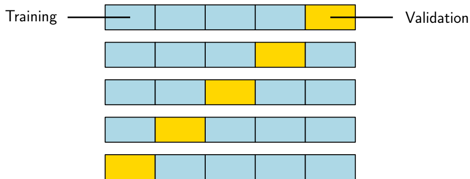
Figure 1.25: K -fold cross-validation. The data set is divided into K = 5 chunks, K - 1 of which serve as the training set (blue) and one as the validation set (yellow). This procedure is repeated for all K choices for the validation set, and the performance of the model from the K runs is averaged.
