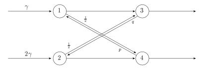
Figure 1: Open queueing network with 4 nodes.
