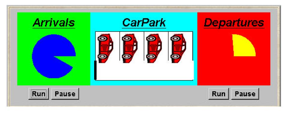
A controller is required for a carpark, which only permits cars to enter when the carpark is not full and does not permit cars to leave when there are no cars in the carpark. Car arrival and departure are simulated by separate threads.
