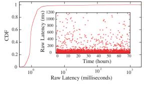
Figure 4. Unfiltered latencies (two nodes)
