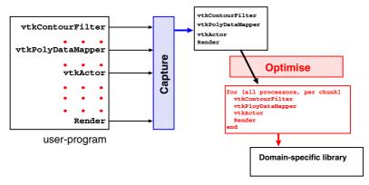
(b) User program is compiled or interpreted by an unmodified language compiler or interpreter. All calls to the DSL are captured and recorded in an execution plan. Domain-specific optimisations are applied to the execution plan before it is executed.
