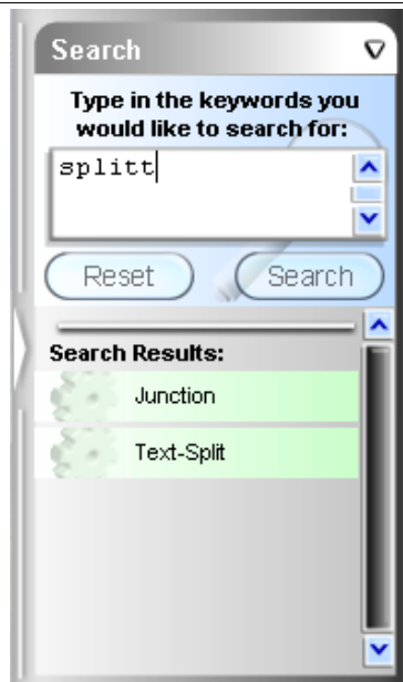
Figure 5.1 An example keyword based search. The user accidentally types in splitt instead of split. The search algorithm locates two matches. Junction is a program for splitting pipes so has split as a keyword. The user can now click each program to get a complete set of information about the program.
