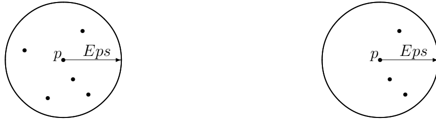
Figure 4.6: Illustration of the density filtering process. Point p remains in the list as the number of points present in N_{Eps}(p) is five (left), and p is eliminated from the list in the case where |N_{Eps}(p)| = 3 (right).
