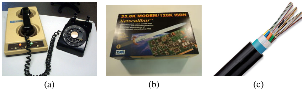
Figure 1.3: Communication technologies: (a) A 300bps acoustic coupler from the 1960s (b) A 128Kbps ISDN modem from the 1990s (Source: Amazon.com and (c) A modern 100Gbps fibre-optic cable (Source: Wikipedia).
