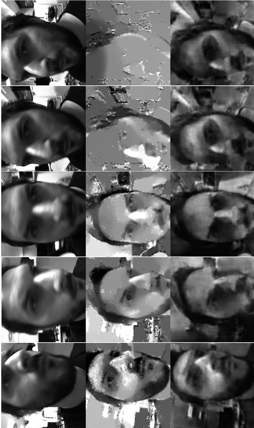
Figure 6.4: Sequence of a moving head, captured by standard camera (first column) and reconstructed by previously proposed method from Chapter 4 (second column) and by our proposed semi-supervised method (third column). Our method can reconstruct much finer details in the background such as the ceiling light which is not visible in the second column and is overexposed in the first column.
