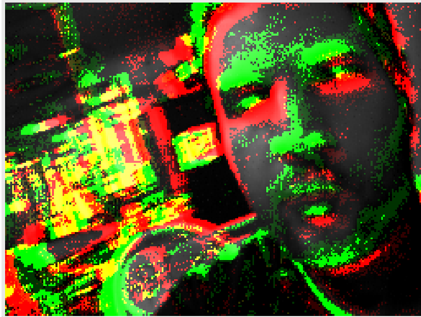
Figure 2.5: Example of the combined output of the DAVIS. The events are superimposed over the monochrome camera image as red and green pixels for positive and negative events. The yellow pixels in the image are regions in which positive as well as negative events occurred.
