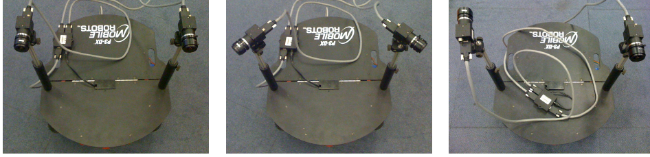
Figure 4.10: The three experimental configurations, with a pair of cameras mounted at relative horizontal angles of 0^\circ , 90^\circ and 180^\circ .
