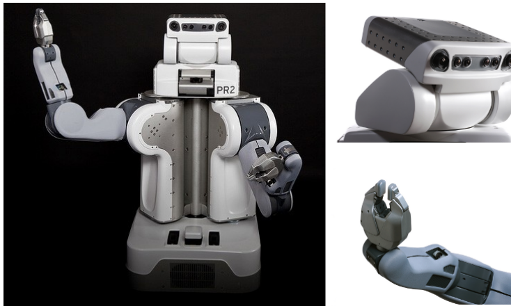
Figure 1.4: PR2 robot from Willow Garage. The vision hardware consists of a Kinect device, two ethernet stereo camera pairs and a high resolution ethernet camera mounted on the head. On the forearm a colour ethernet camera is also mounted.
