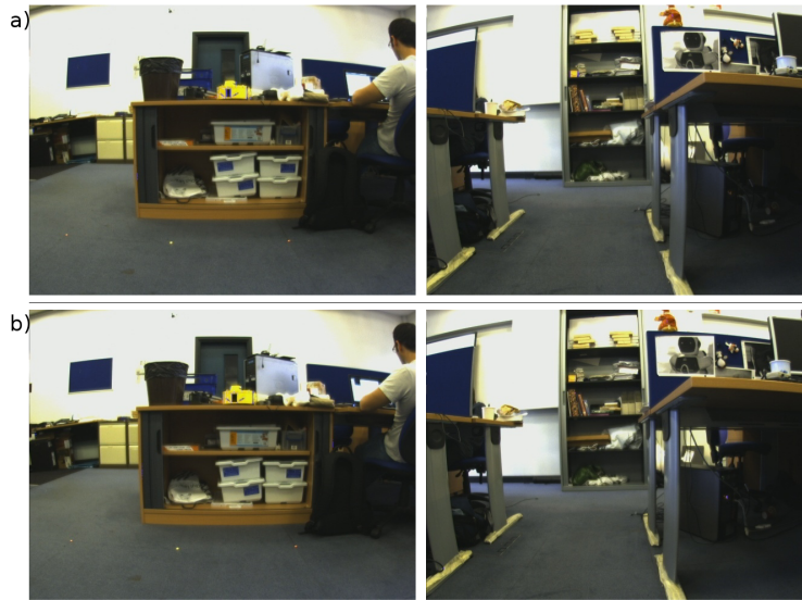
Figure 6.3: Loop closure detection with a forward and backward camera configuration. The top image shows the current image at time t , the bottom shows the best match found over the previous keyframes at time t - k . Where k is the number of keyframes in the history of the robot's trajectory.
