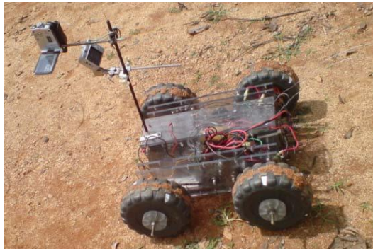
Figure 7.10: Skid steered robot [106] : two cameras are used on a robot to compute VO: one facing to the floor, the other facing forward.
