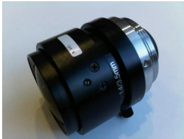
Figure 3.9: Lens used in our cameras, Model L-SV-03514: 3.5mm, F1.4 CCTV, 1/2in format, C- mount, HAV of c.80deg for 1/3" sensor.
