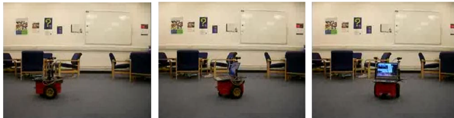
Figure 4.5: Images of the robot performing a pre-programmed motion for the camera rig calibration procedure.
