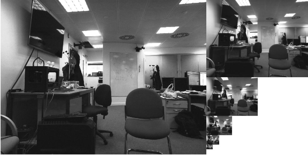
Figure 2.3: A Gaussian pyramid with 6 levels created from the live image for tracking
