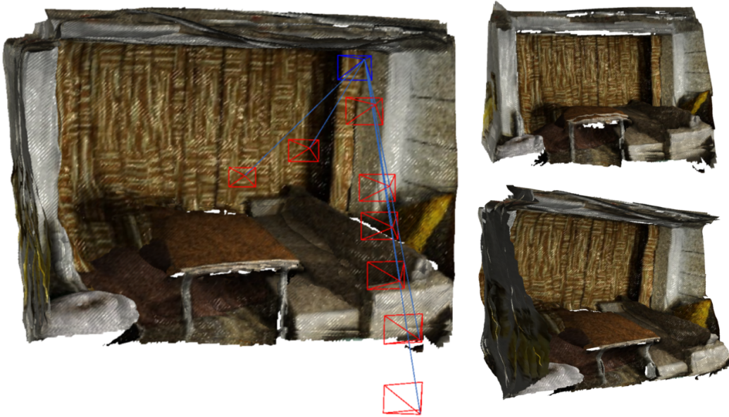
Figure 4.11: Monocular 3D reconstruction using 9 keyframes. During optimisation a selected master keyframe is paired with the other frames. The depth images of all frames are used for the 3D rendering. The employed geometric error term ensures the consistency between the depth of the different views.
