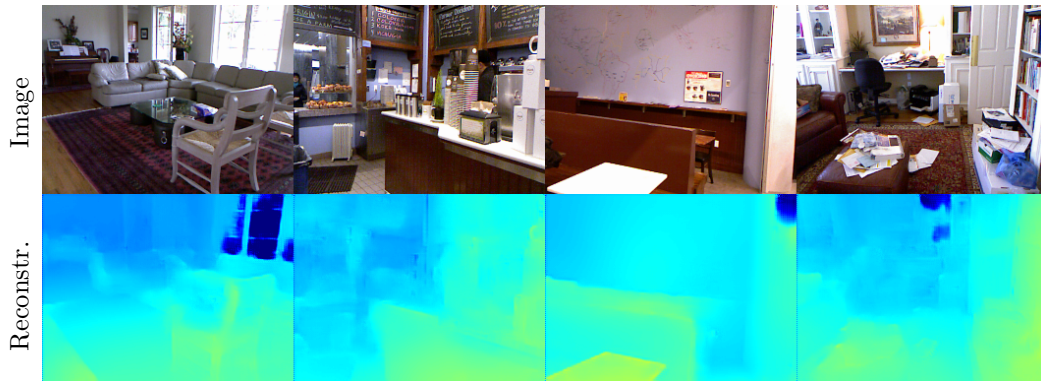
Figure 4.12: Two-frame SfM on selected pairs from the NYU V2 dataset. Top row presents one of the images used for reconstruction, while the bottom row contains respective depth estimates. The main elements of all scenes can be well perceived in the depth image. The overexposed image regions saturate to infinite depth values, which is a result of using the SceneNet RGB-D dataset for training, which contains many scenes with windows (similar to the one in the left image).
