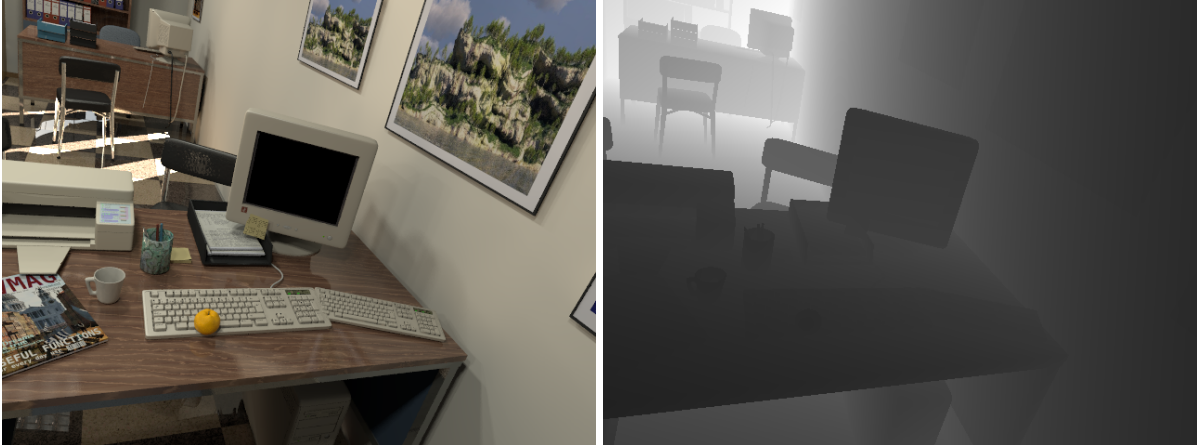
Figure 5.11: A ‘pure’ ray-traced image with no blur or noise effects. Each such image takes 30–60mins to render in two passes on an 8 core Intel i7 3.20GHz machine. The associated planar depth map also generated is shown alongside.
