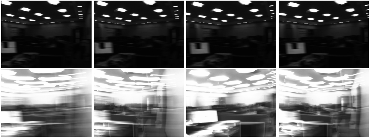
Figure 7.9: Consecutive images obtained at 200Hz (top row) and 20Hz (bottom row) for this motion. Such fast motion introduces motion blur even at 200Hz which is more evident on the monitor screen. Far more importantly, low frame-rates e.g. 20Hz not only have significant motion blur but also large displacement which makes it hard to register images and often leads to tracking failures at these frame-rates.
