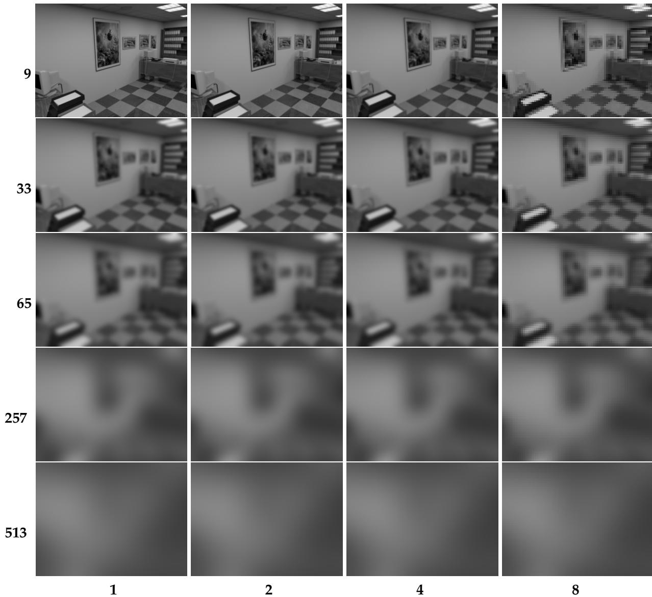
Figure 6.13: Sample image shown with progressive increase in the amount of blur with their pyramidal levels. The vertical axis reads the kernel size and horizontal axis, the subsampling factor of image. Such blurring could appear in the case of camera defocus. In all the experiments the depth-map was blurred by the same amount. Tracking performs without breaking even at 257 \times 257 kernel size.
