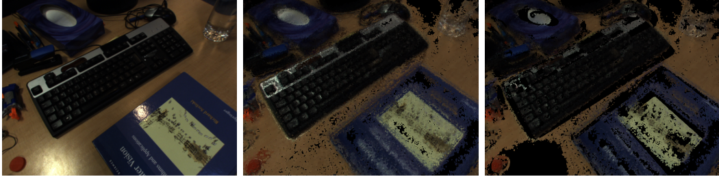
Figure 6.4: Outlier removal. The rendered model image (middle) is compared to the camera image (left). Pixels that are inconsistent are removed (right). Removing the outliers can make tracking more robust. Specularities, such as on the table in the bottom left of the images, are a typical occurrence which are removed by this processing.
