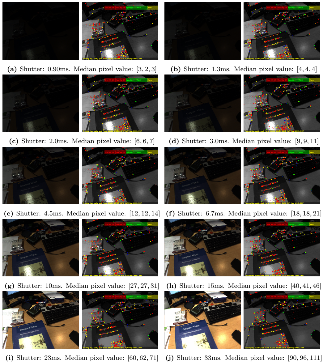
Figure 3.11: The shutter time of a handheld camera is varied on every frame yielding images with massive changes in exposure (left). The images are renormalized to a fixed exposure (right) and PTAM is still able to track the camera robustly. In image (a) a human cannot see any information in the image but when renormalized there is actually plenty of detail for PTAM to track against. The renormalized image has much more noise but still not enough to break tracking. The median pixel value of the raw camera image is provided to give a quantitative measure of exposure.
