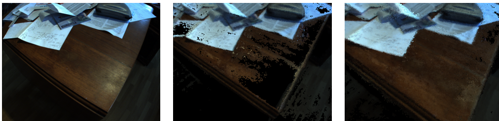
Figure 6.13: The specularity on the lower right corner of the table (left) prevents the surface from being reconstructed (middle), resulting in a hole. However, with a change of viewpoint we are able to reconstruct the surface from views where there is no specular component (right).
