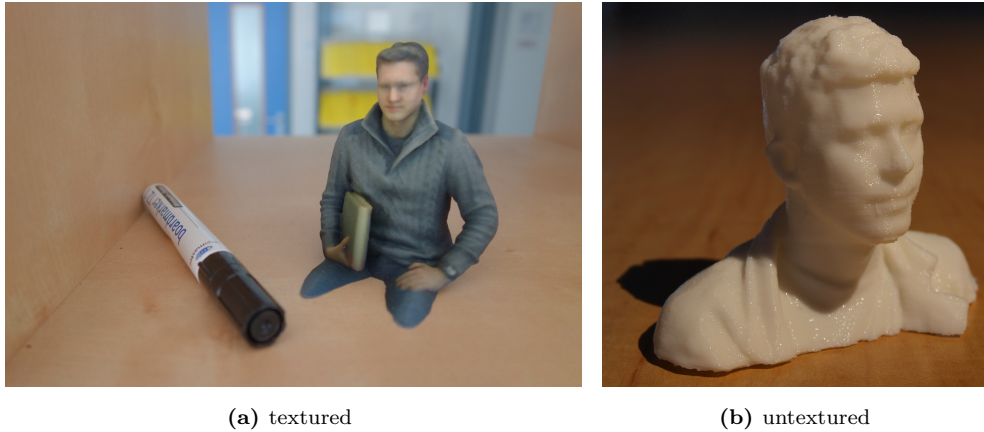
Figure 4.3: (a) Commercial 3D printing services offer the ability to produce a textured model [42]. The texture is able to hide inaccuracies and low quality geometry. (b) The majority of consumer 3D printers are only able to print in a single colour, much like traditional sculpture.
