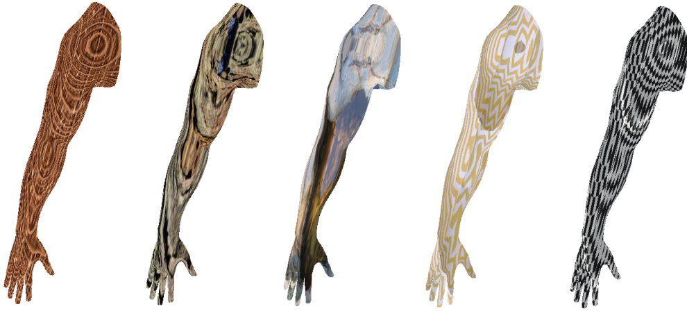
Figure 5.11: An example of the variations we get when we apply domain randomisation to the simulated human arm.
