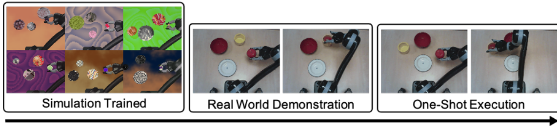
Figure 5.1: The robot gains its few-shot learning ability in simulation, and can then learn a new task from a single demonstration.
