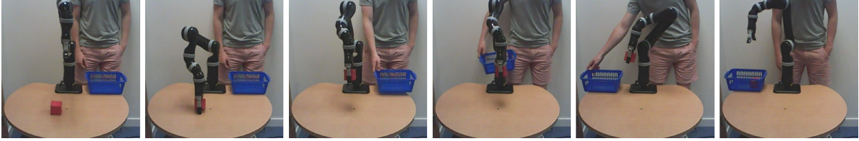
Figure 3.5: A sequence of images showing the network’s ability to generalise. Whilst a person is standing in the view of the camera, the robot is able to grasp the cube and proceed to the basket. As the arm progresses towards the basket, the person moves the basket to the other side of the arm. Despite this disruption, the network alters its course and proceeds to the new location. During training, the network had never seen humans, moving baskets, or this particular table.
