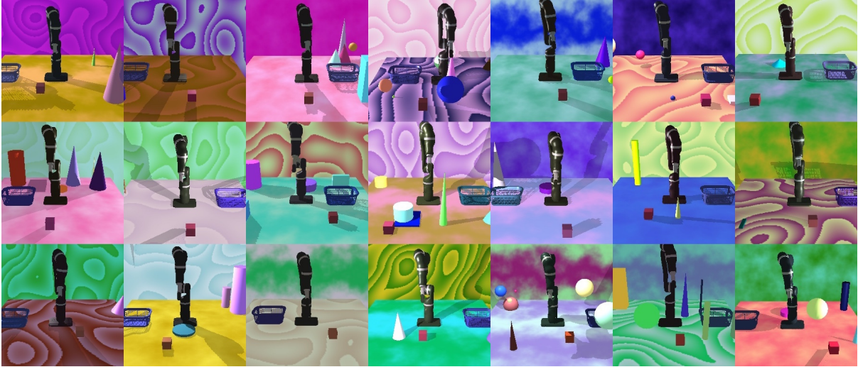
Figure 3.2: A collection of generated environments as part of our domain randomisation method.
