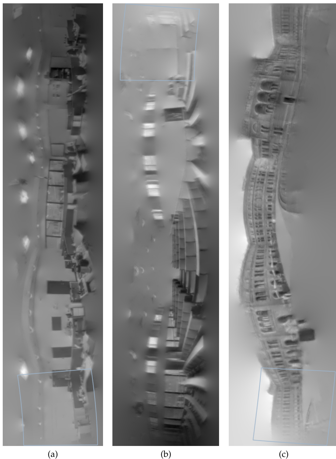
Figure 4.10: Reconstructed spherical mosaics for indoor (shown in (a) and (b)) and outdoor (shown in (c)) scenes with super resolution and high dynamic range properties — converted to intensity values for visualisation purposes. The overlaid boxes represent the current field of view of the event camera being tracked.
