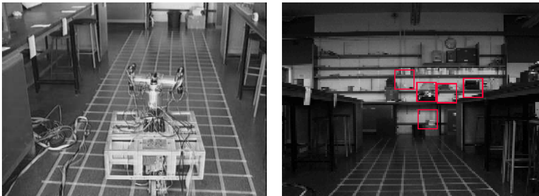
Figure 1.1: One of the first full joint EKF-based real-time visual SLAM system which navigates in unknown environments by tracking selective sparse landmark features with an active stereo camera on a wheeled robot, showing a highly constrained and hardware-dependent setup in the early period of the visual SLAM research. Figures courtesy of Davison et al. [40].
