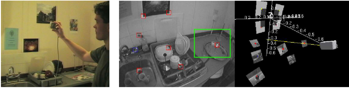
Figure 1.2: MonoSLAM was one of the first real-time monocular SLAM methods which tracked 6-DoF hand-held camera motion while building a sparse set of features based on a sequential probabilistic filter showing the most general and simplest setup in visual SLAM. Figures courtesy of Davison et al. [42].
