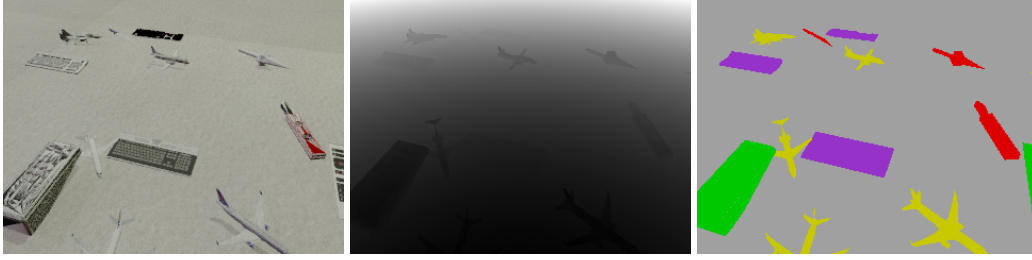
Figure 4.16: Dataset example from the view-based dataset. Left to right: RGB, depth and pixel-wise semantic annotation.
