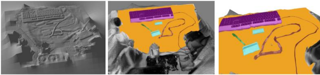
Figure 4.9: Left: reconstructed height map of a table top scene. Centre: the corresponding intensity image, with label annotations. Right: A screenshot of the 2.5D Semantic ground truth height map after loading the annotated height map back into height map fusion.
