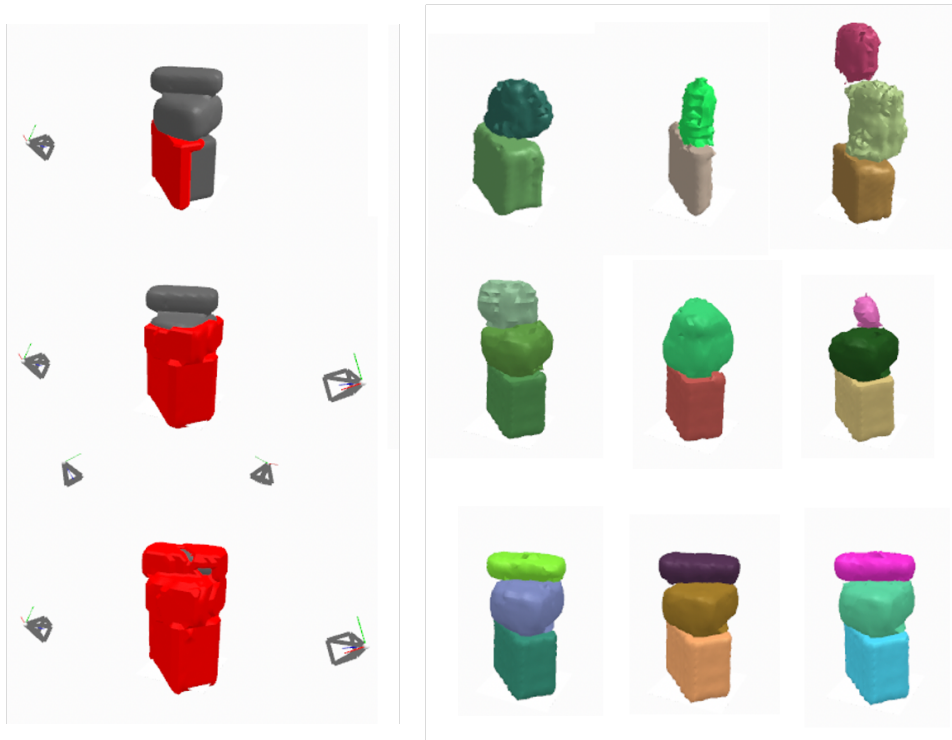
Figure 5.38: How sampling variety changes as views are added. Left: Ground truth and visible mesh area overlay (red). Right: 3 random latent space samples (without SQ fitting) for each view; as data is added the samples are increasingly constrained.
