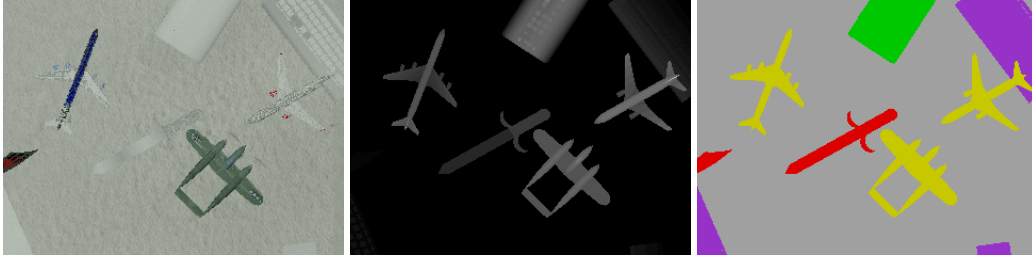
Figure 4.17: Dataset example from the map-based dataset. Left to right: RGB, height (inverse depth) and pixel-wise semantic annotation. The presented images are cropped sub-samples from a larger height map reconstruction.
