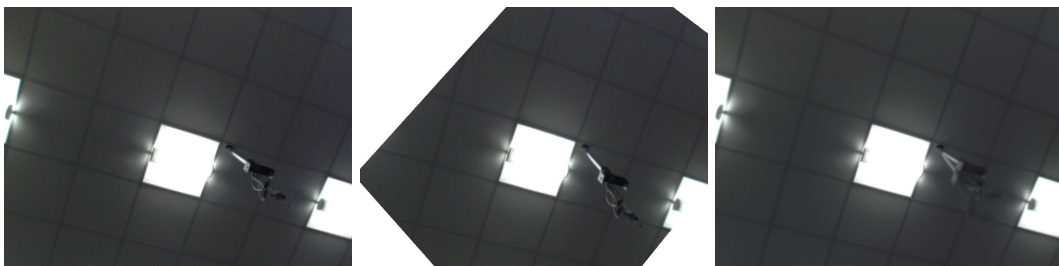
Figure 5.21: Planar Mosaic (right) generated from multiple keyframes (e.g. left, middle) where planar assumption is not strictly true. Mosaic generated by blending constituent keyframes with equal weight.
