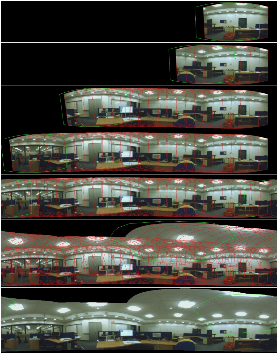
Figure 5.4: A mosaic is constructed incrementally, estimating camera pose live but saving sparse historic video frames when the overlap with the current mosaic drops below a threshold. Keyframes are shown outlined in red. Loop closure can be seen to tighten the map after a full 360 degree trajectory has been closed.
