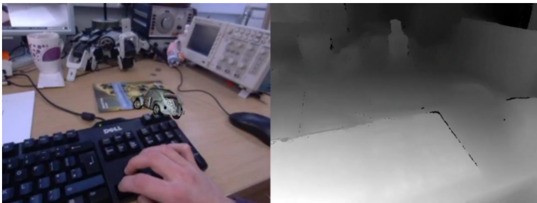
Figure 6.12: The dense surface model can be used for augmented reality, offering a depth map for the live camera view and a rigid mesh with which physical models can interact.
