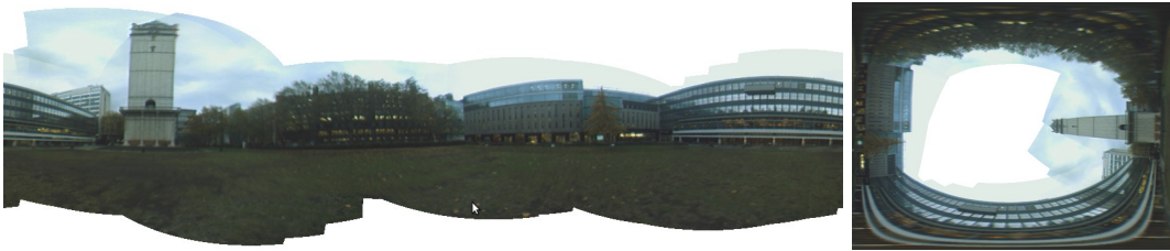
Figure 5.15: 360^\circ Tower panorama from 21 keyframes (live hand held Unibrain webcam, 320 \times 240 resolution), shown in horizontally and vertically-oriented cylindrical projection. Note the vertical hole due to poor texture and cloud movement in the sky.
