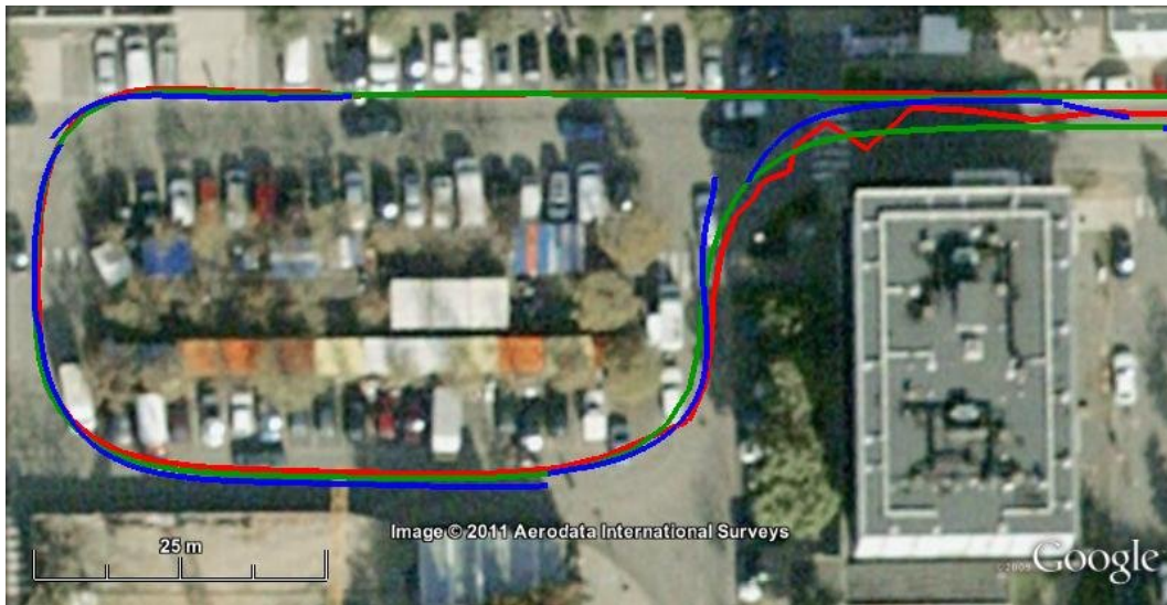
Figure 4.13: Four 10 second sequences of integrated visual odometry (blue) against GPS (red) and ground truth (green).
