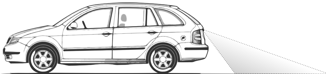
Figure 4.7: A rear parking camera, as fitted to many current vehicles, views the road surface directly behind the car during normal driving.
