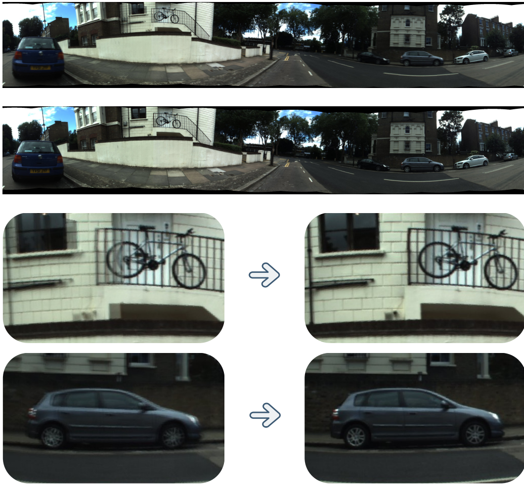
Figure 5.14: Mosaicing with (middle) and without (top) live intrinsic refinement. Enlargements of these mosaics are shown (bottom) highlighting the improved registration as error is propagated more accurately throughout the 360 degree trajectory.
