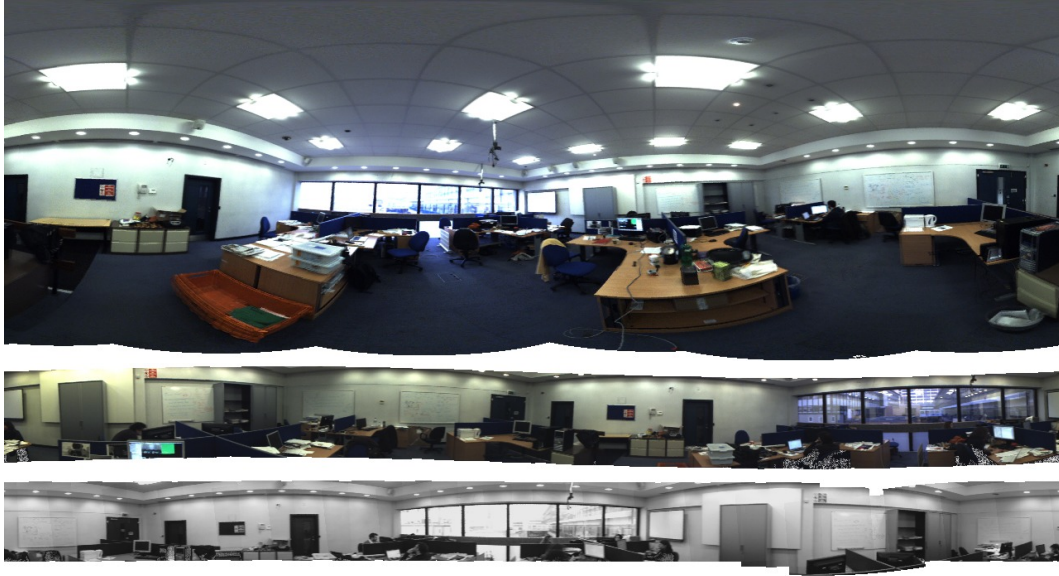
Figure 5.12: 360° spherically-projected panoramas for three indoor sequences, taken with different lenses. Point Grey Flea2, 70° FOV wide angle (top, close to full sphere including full hemispherical upward coverage, 27 keyframes), 50° FOV TV Lens (middle, single horizontal loop trajectory, 17 keyframes), and Unibrain 45° FOV Standard lens (bottom, single horizontal loop trajectory, 19 keyframes).
