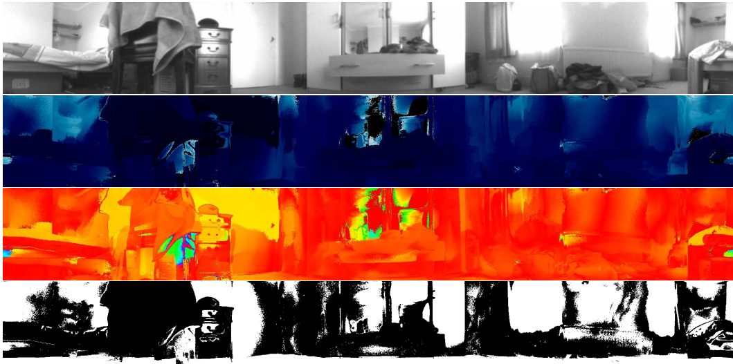
Figure 6.31: Dataset “Wandsworth Bedroom 3”, from top to bottom: reference frame, estimated depth map, depth map error, depth threshold mask.
