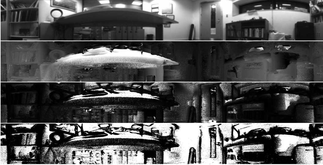
Figure 6.2: Dataset “Cluttered Office”, from top to bottom: reference frame, estimated depth Map, estimated depth standard deviation map, depth threshold mask.
