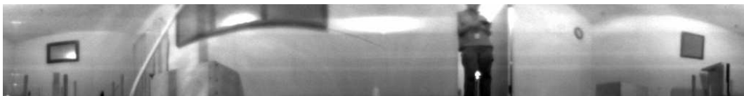
Figure 3.2: Optical artifacts from a low-cost omnidirectional lens.
