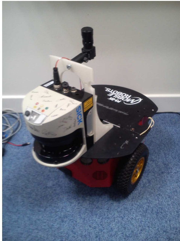
Figure 4.3: Robot equipped with a planar laser scanner.
