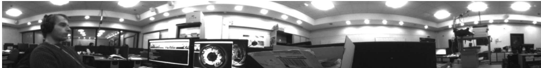
Figure 3.8: Panoramic unwrapping with LUT performed by the GPU
