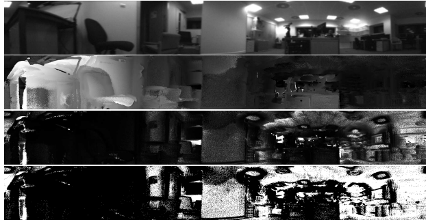
(a) Dataset “Large Office”, one of the measurements, from top to bottom: reference frame, estimated depth map, estimated depth standard deviation map, depth threshold mask.
