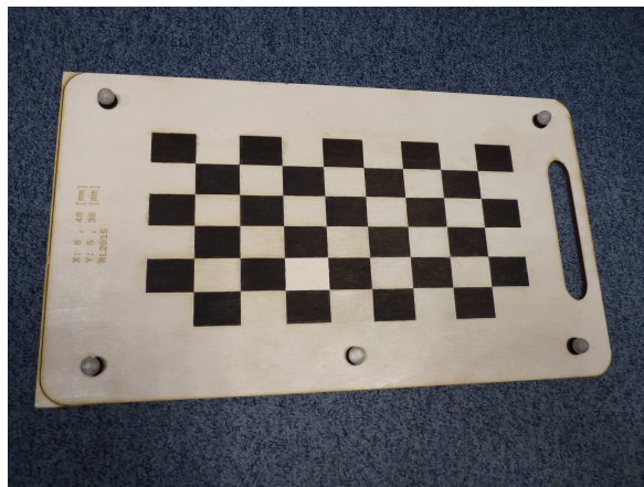
Figure 4.5: Combined vision and ground truth tracker calibration pattern.
