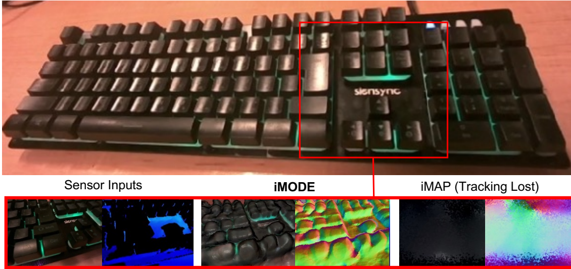
Figure 3.11: Small-scale reconstruction: While commodity depth sensors cannot measure surfaces closer than 10cm and iMAP completely fails at this scale, our purely monocular system can reconstruct each key of the mechanical keyboard.
