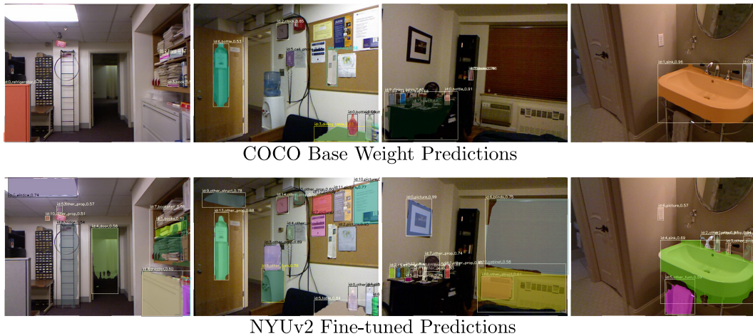
Figure 6.9: Qualitative comparison of the Mask R-CNN instance predictions on the NYUv2 test using the base COCO trained weights (top row) and predictions after fine-tuning on the NYUv2 training set (bottom row). Predictions with confidence > 0.5 are shown. Fine-tuning improves the recall of smaller objects.
