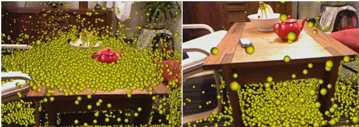
Figure 9.24: Thousands of particles interact live with surfaces as they are reconstructed. Notice how fine-grained occlusions are handled between the real and virtual. Simulation works on the TSDF volumetric representation, and runs on the GPU alongside tracking and mapping, all in real-time.
