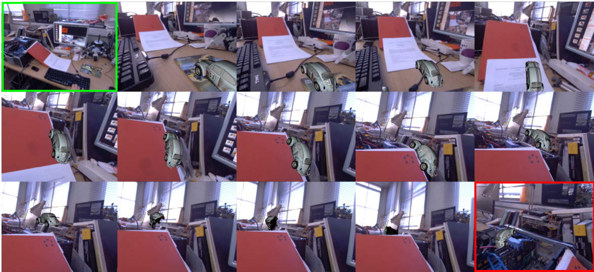
Figure 9.14: Example geometry aware augmented reality with a car. Completing the scene reconstruction shown in Figure (9.13), the dense surface model is used in an augmented reality game enabling the desktop to be driven over by a virtual car with simulated physical interaction over the static scene. We show an overview of the scene that is reconstructed in the top left corner of the figure (green box), and illustrate the large scale over which dense tracking with the model is performed: following the virtual car with the live camera as it drives up a ramp constructed from a book, and coming to stop atop of the graphics card currently running the DTAM computations (bottom right, red box).
