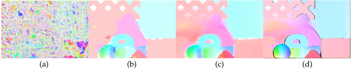
Figure 5.8: Coloured flow fields for the rubberwhale two view optical flow data set: Single pixel data term minimum (a); regularised exact search on integer flow vectors (b); regularised exact search with embedded interpolation using Equation (5.25), demonstrating sub-pixel flow solution without the additional computational cost in explicit data term oversampling (c); ground truth flow field (d), ground truth flow field and colouring scheme from (Baker et al., 2011).
