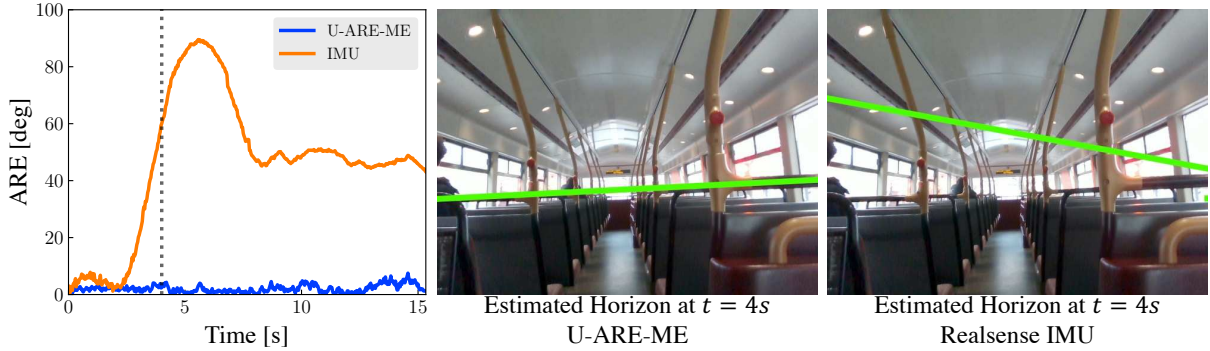
Figure 7.6: IMU sensors are prone to drift especially in non-inertial frames of reference (e.g. inside a moving vehicle). The horizon line in each image represents the up-vector inferred from our proposed method (middle) and an IMU sensor (right).
