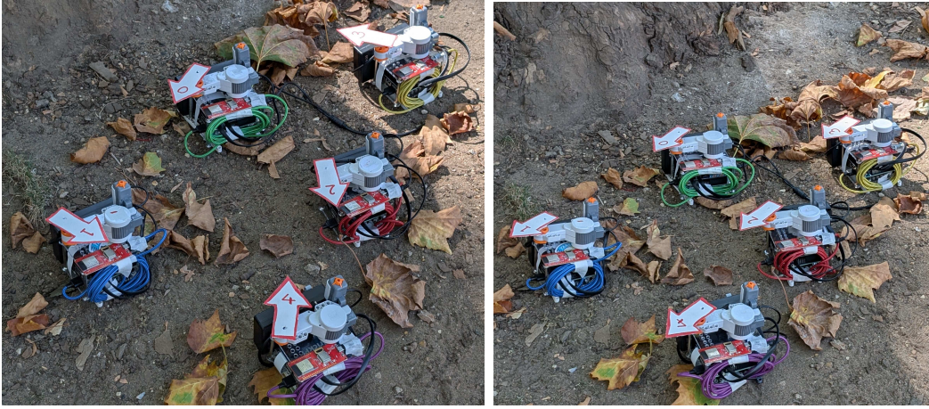
Figure 6.9: Multi-robot consensus demonstration in the wild. 5 devices are initialised with prior angles \mathbf{z}_d \in \text{SO}(2) indicated by their arrows (left). When the devices switch on, they create inter-device factors with their neighbours and achieve consensus on a global direction to point towards (right). Using the ESP-NOW protocol removes the need for a central WiFi network for communication and control.
