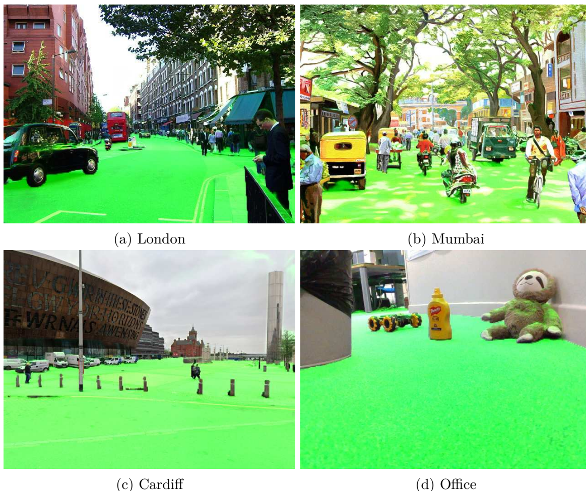
Figure 7.7: Even in non-Manhattan scenes, our framework can optimise the rotation such that the global up direction is aligned with the surface normal of the ground plane. It can thus be used to accurately segment the ground plane, shown here in green, which can be useful for many applications in robotics.
