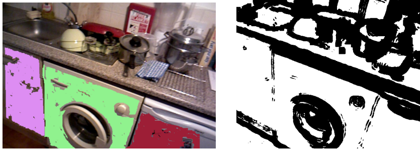
Figure 6.4: Planar region detection. (left) Three planes have been detected with connected component labelling using the measured vertex and normal maps. (right) A depth discontinuity map is used to avoid labelling regions with low quality normals (black pixels).
