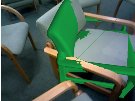
Figure 3.3: A scene with a nearby object before ICP alignment. The colour scene represents the data surface, while the green object is the model .
