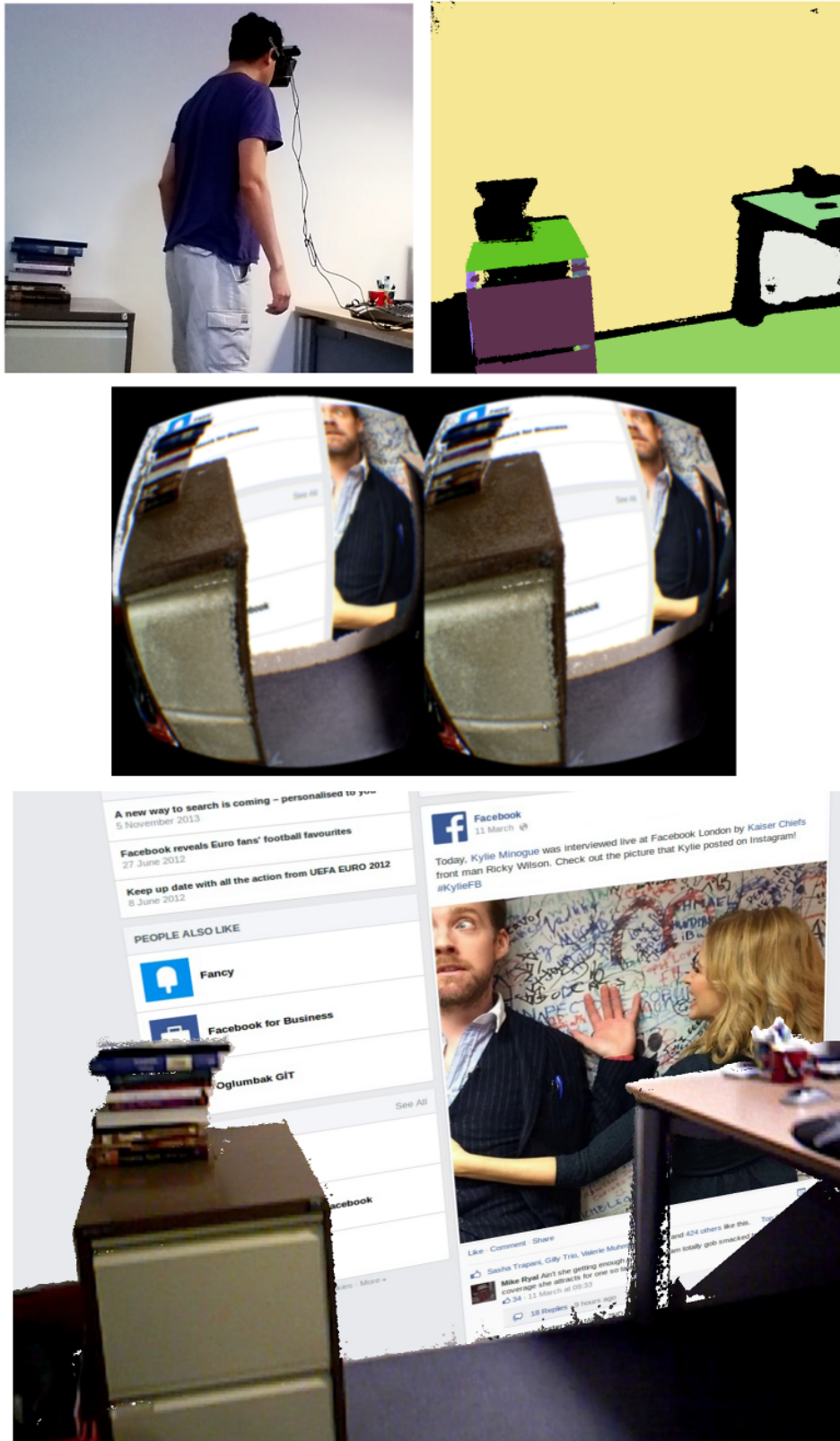
Figure 6.11: Facebook Wall on a real wall using the Oculus Rift. The user chooses a wall from which to read his Facebook Wall.
