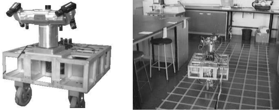
Figure 1.1: Robotic platform used in the active vision SLAM work of Davison et al. [36] in 1998. © Andrew Davison.
