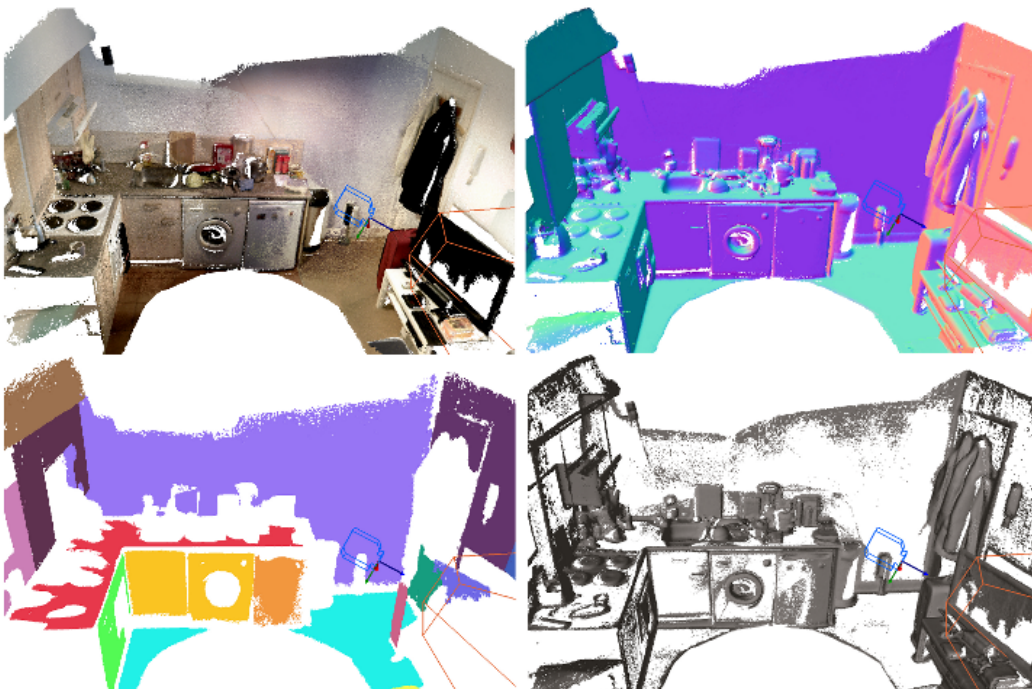
Figure 6.9: Real scene reconstruction of an apartment. (top) Displaying both planar and non-planar regions surfels. (bottom) In clockwise order: Colour output, Normal Map, Non-Planar region surfels only, Planar region surfels only.
