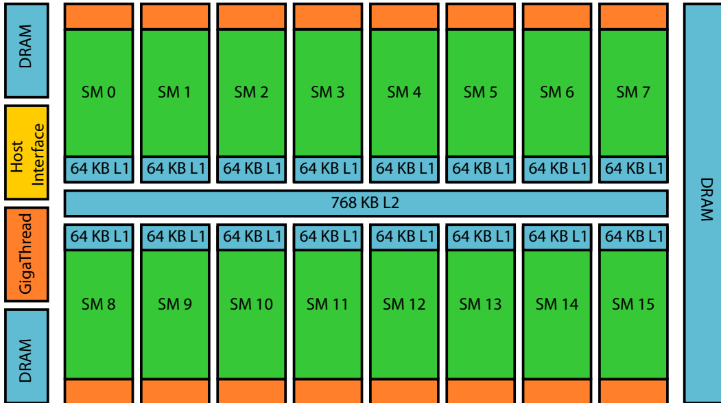
Figure 3.5: The Fermi GPU architecture. A set of 16 Streaming Multiprocessors (SM) execute parallel operations organised by the GigaThread global scheduler. Each SM contains a local configurable L1 memory while fast GPU-wide caching is achieved via a L2 cache. Adapted from [164].
