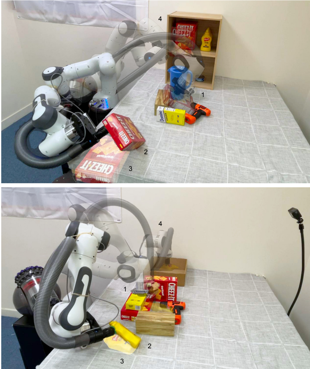
Figure 5.1: ReorientBot , our manipulation system for object specific-posed placement, picks, reorients, regrasps, and places objects in various target configurations. Learned components enable object reorientation with significant rotation using dynamic placement (released and stabilized with gravity), which is hardly achievable with human heuristics.
