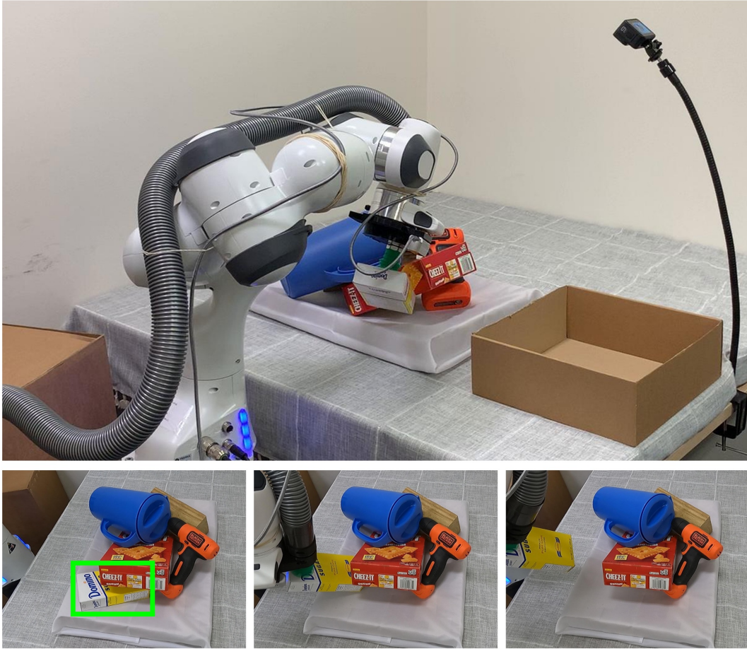
Figure 4.1: SafePicking , our manipulation system for object extraction, extracts target objects with minimum disturbance by generating a safe end-effector trajectory given raw observations and object poses retrieved from an object-level semantic map.
