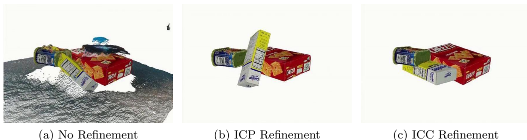
Figure 3.7: Pose refinement from intersecting object poses , where we compare the Iterative Collision Checking (ICC) against Iterative Closest Point (ICP).
