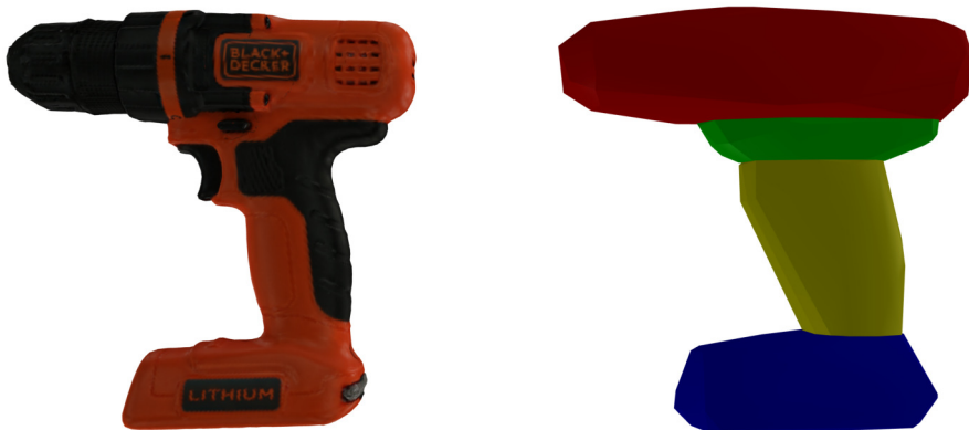
Figure 2.7: Convex decomposition of a mesh model for collision detection.
