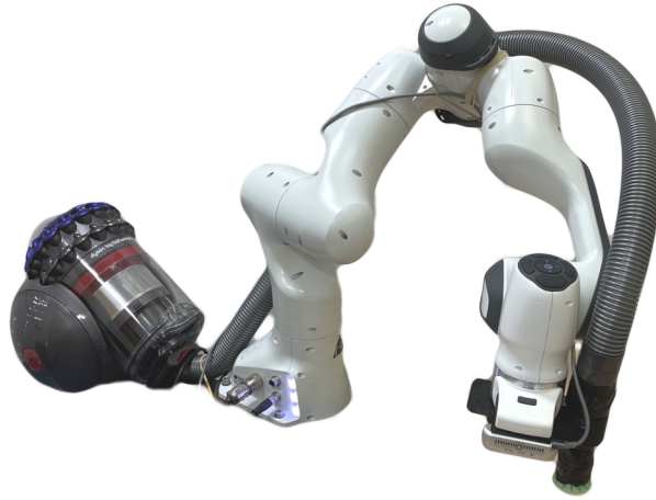
Figure 2.6: Franka Emika Panda robot that we use in our experiments with the custom suction gripper with a vacuum cleaner.
