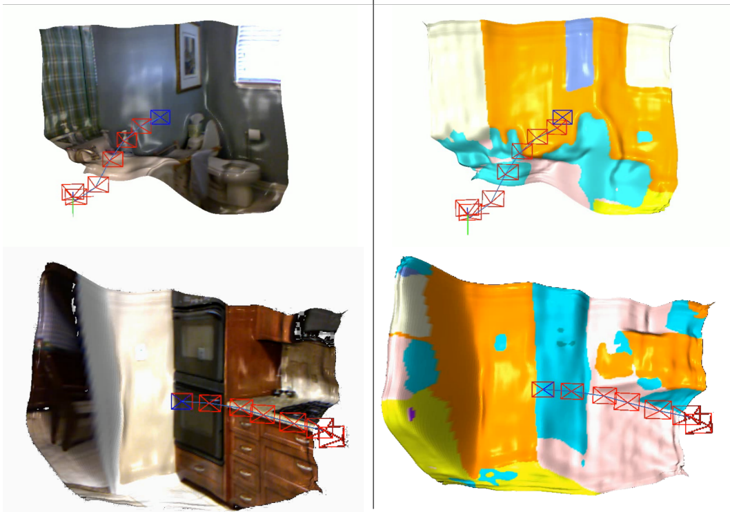
Figure 3.14: Qualitative result of monocular dense semantic SLAM system in bathroom and kitchen sequences of the NYUv2 dataset.
