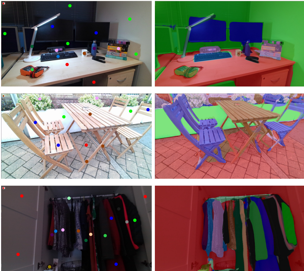
Figure 5.6: Ultra-efficient label propagation: iLabel produces high-quality segmentations of coherent 3D entities with very few user clicks, approximately 20–30 per scene.
