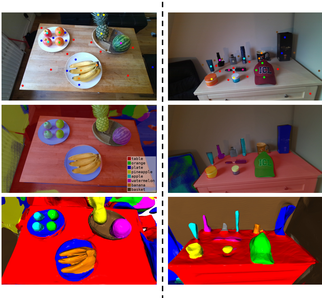
Figure 5.5: Precise segmentations can be obtained from just 1 or 2 clicks per object. From top to bottom are keyframes with user clicks, rendered 2D segmentation and semantically annotated 3D mesh, respectively.
