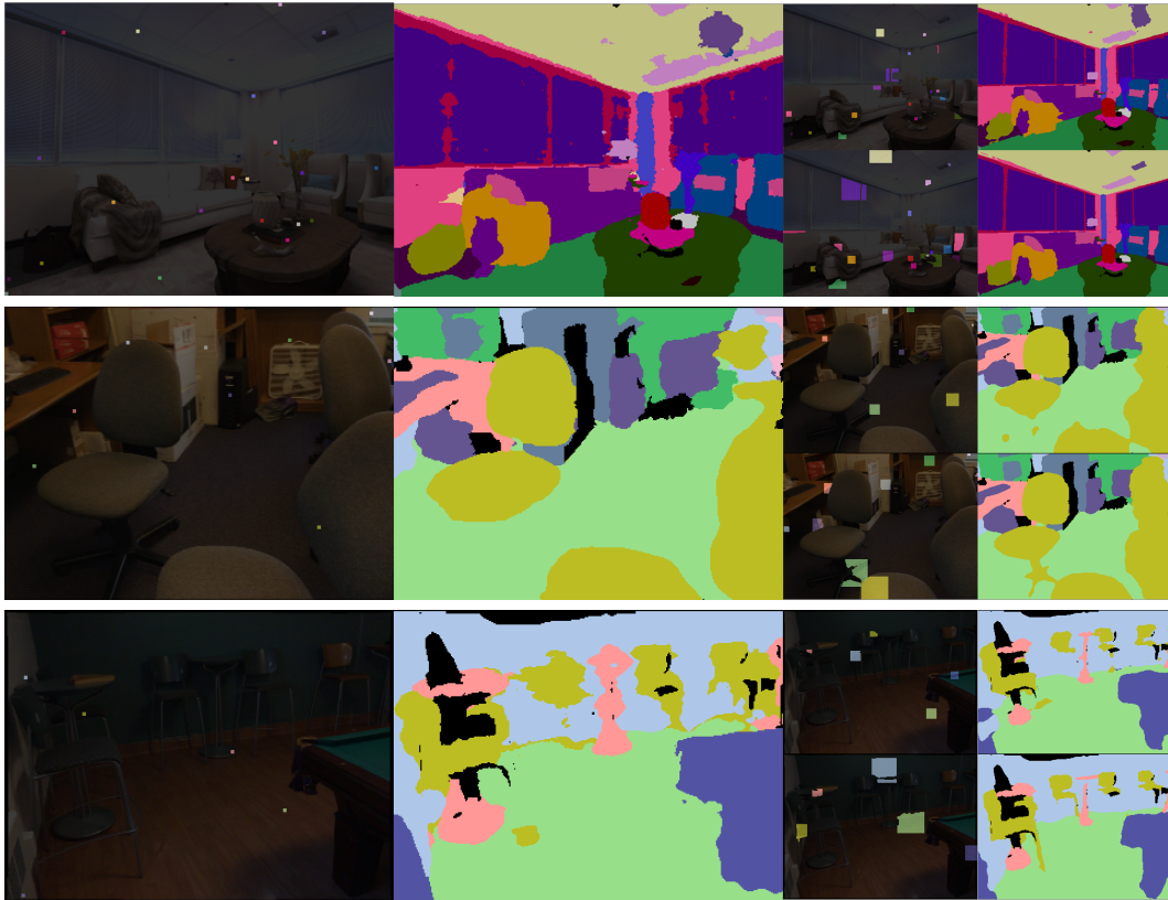
Figure 4.10: Label propagation results using partial annotations of a single-pixel, 1% or 5% of pixels per class within frames, respectively. Accurate labels can be achieved even from single-clicks, which are zoomed-in 9 times for visualisation purposes.
