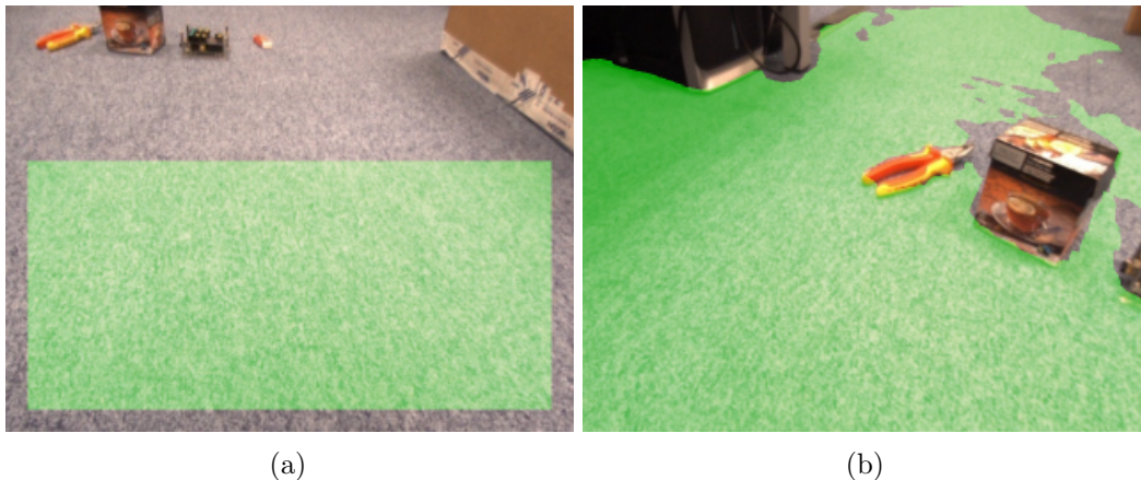
Figure 3.5: Our method does not require that all pixels in the camera field of view belong to the planar floor, and in practice we perform dense image alignment on the image parts that are confidently identified as a planar floor. We start by assuming that only the area directly in front of the robot is planar (a). This is sufficient to perform accurate motion estimation, and allows us to estimate depth maps (Chapter 2) that next can be used to classify pixels into ‘floor’ and ‘non-floor’ (b), by for example building appropriate appearance models [Dahlkamp et al., 2006; Hadsell et al., 2009] or performing a surface reconstruction as shown in Chapter 6.
