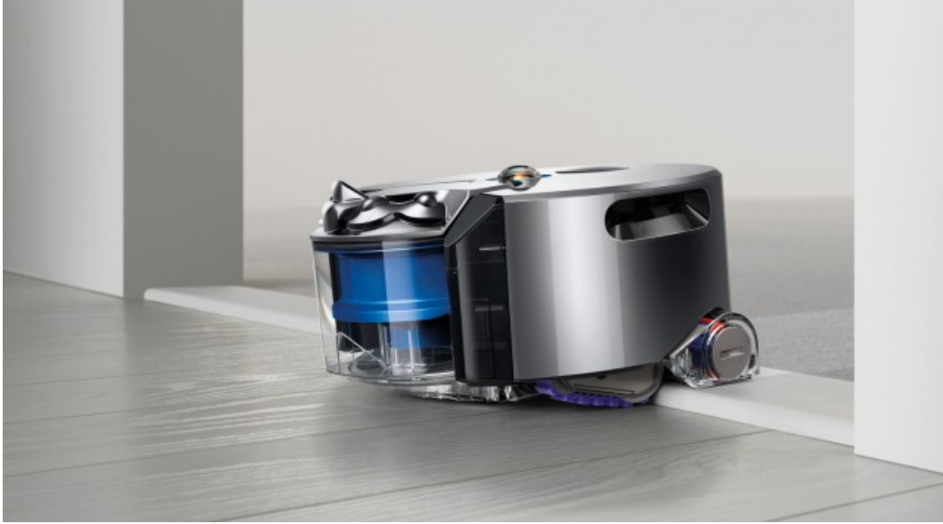
Figure 1.1: The Dyson 360Eye™ robotic vacuum cleaner and similar domestic robots are motivating examples for our study in which we address the question of whether a single camera can provide a mobile robot with enough capabilities to perform autonomous navigation and mapping. (Image reproduced courtesy of Dyson.)
