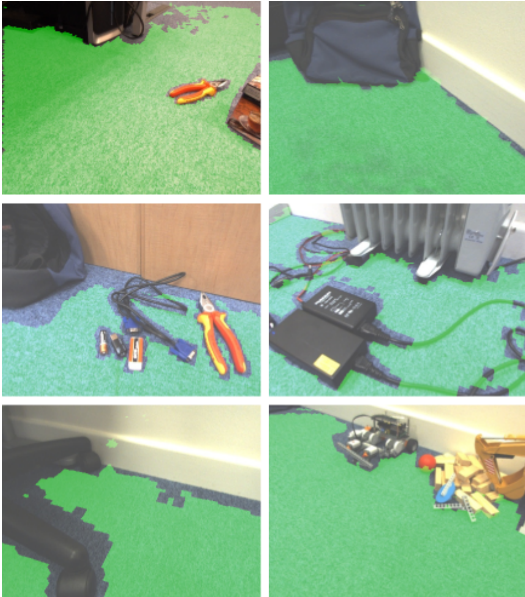
Figure 6.8: Free space detected (green overlay) by simple thresholding of the reconstructed elevation map.
