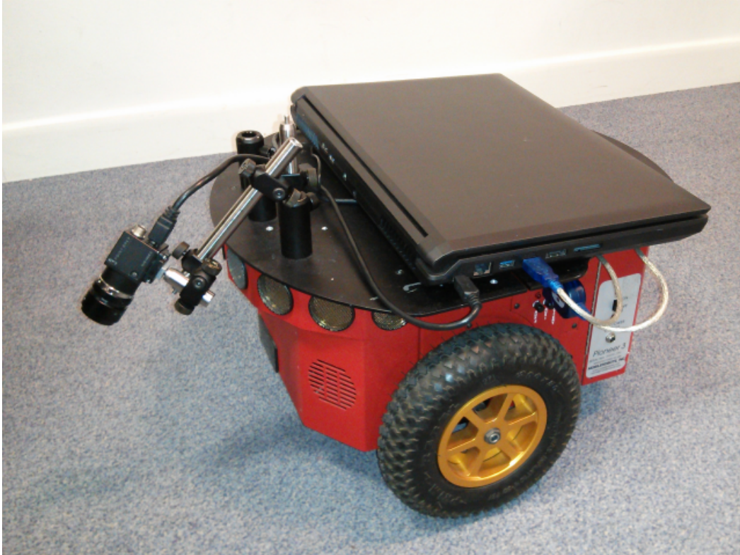
Figure 3.6: Robot Pioneer P3-DX used for in our experiments.
