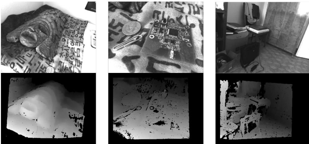
Figure 2.9: Our method can estimate depth maps in real-time also in more general settings, when paired with 6 DoF tracking such as ORB-SLAM.
