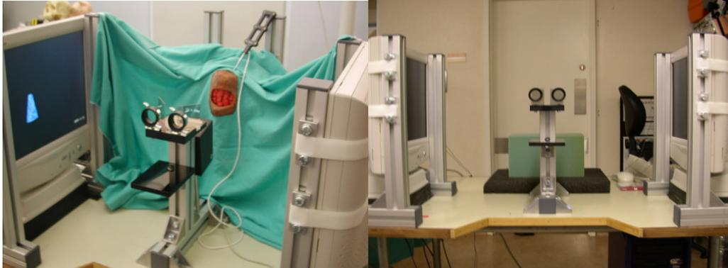
This system was intended as a test-bed for perception in stereo AR. Though MARS is anything but miniature, it provides one of the most compelling 3D AR experiences.
