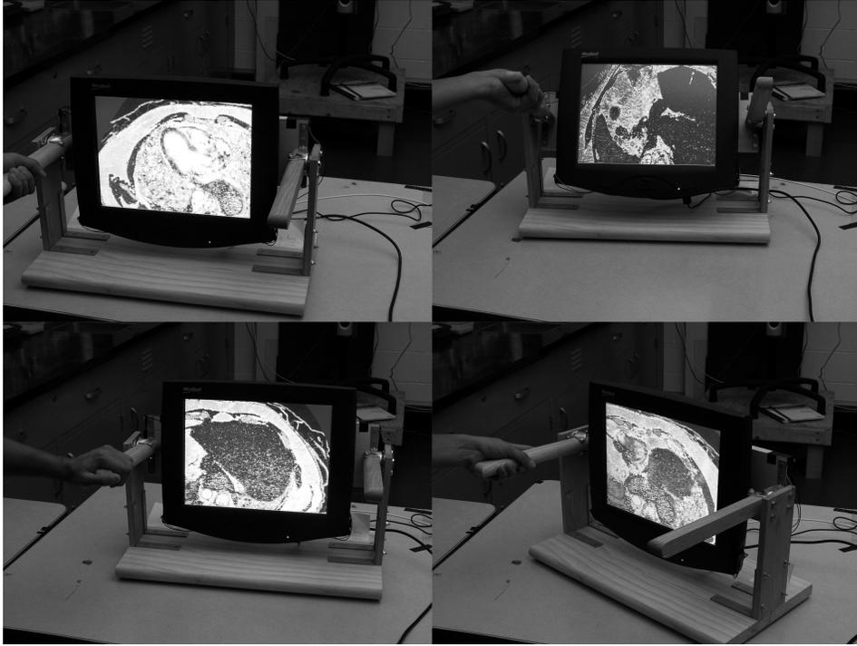
**Fig. 2.** The grab-a-slice display showing CT images of the lung. Various locations and orientations of the display result in corresponding slices through the invisible patient being displayed. Degrees of freedom consist of 2 translations and 2 rotations.
