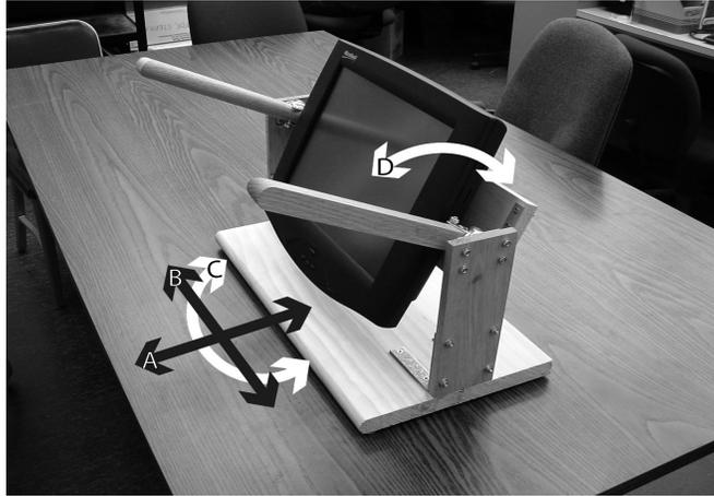
**Fig. 1.** The current grab-a-slice display can be manipulated in four degrees of freedom (see text).
