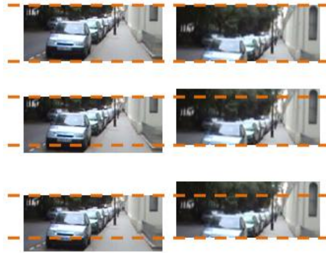
Figure 3.10: Sub-image of frame t+1 is shifted vertically until it is matched with frame t in the best possible way
