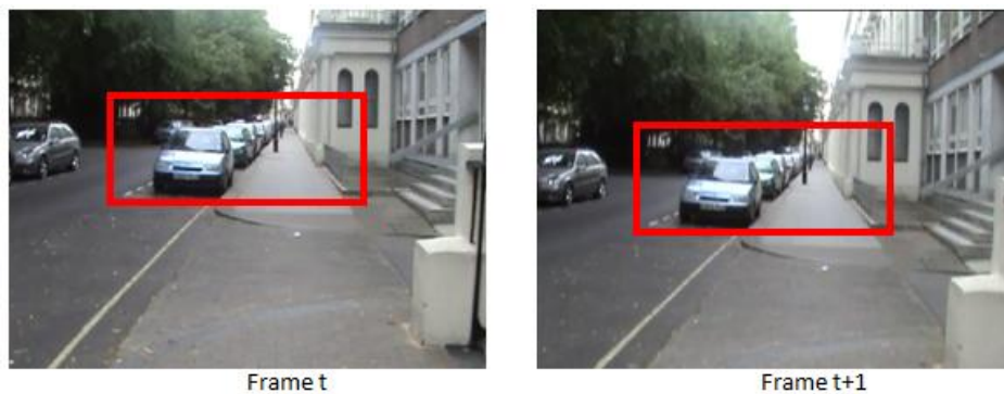
Figure 3.11: Frame t+1 is assigned a new, corrected sub-image, which is then sent to the visual odometry module
