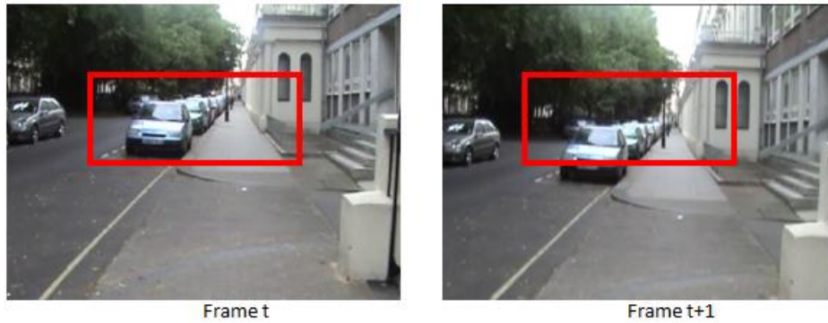
Figure 3.9: Two consecutive image frames, with sub-images selected for the visual odometry module.
