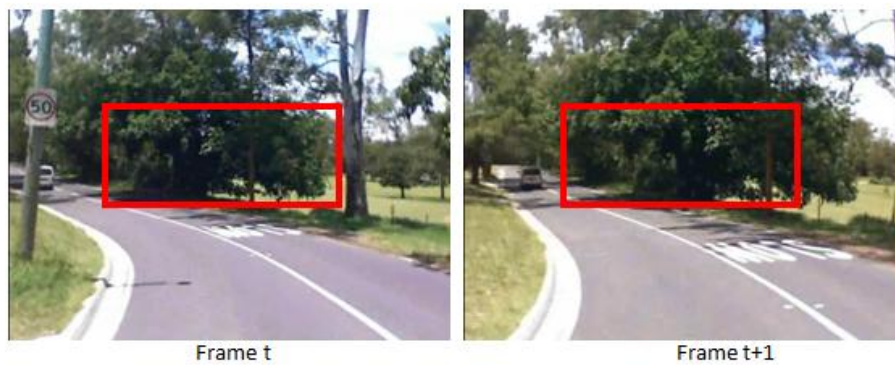
Figure 3.7: Consecutive frames captured by a stable camera. The inner squares, are the subsections the visual odometry module extracts for calculating rotation. The sum of absolute differences based on pixel intensities is then calculated in a per column pattern
