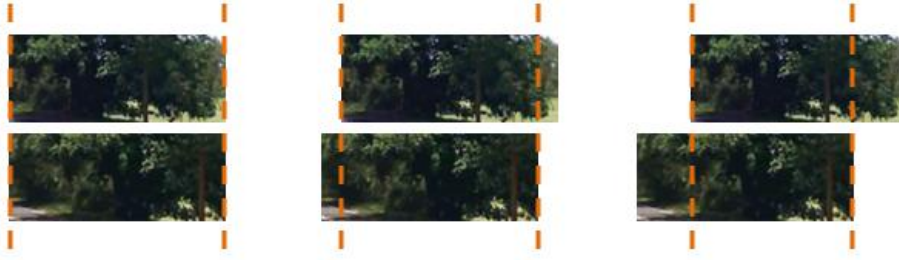
Figure 3.8: Shifting Frame t+1 to the left, until the sum of absolute difference in intensities between the two images is minimised
