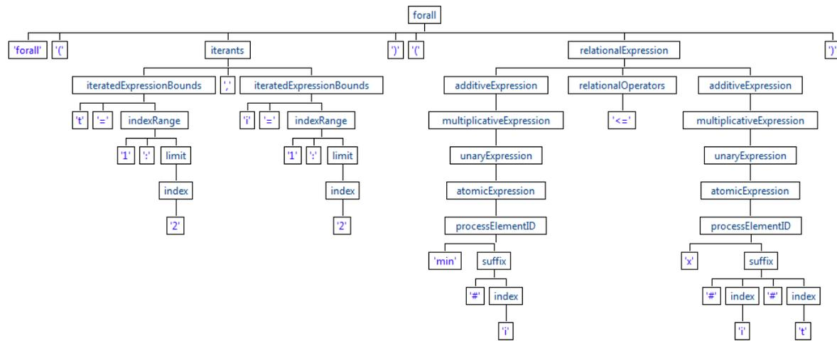
Figure 6.2: Diagram showing the interpretation of the *universal quantification* parser rule for code listing 6.5 (line 4).
