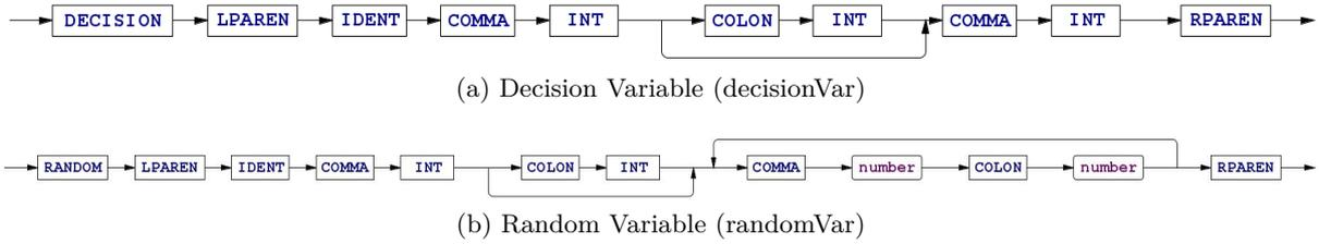
Figure D.3: Syntax diagrams representing the extended context-free grammar specified in the JADAParser source file for the *Variables* language construct.
