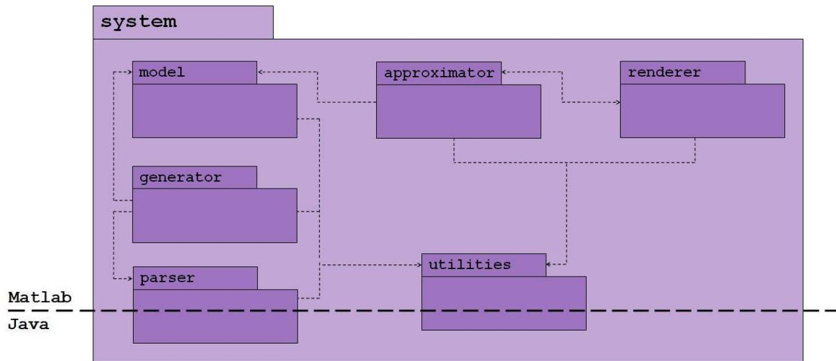
Figure 5.1: UML diagram showing the package structure, where the dashed arrows indicate the package dependencies. The separation between the Java implementation and MATLAB implementation is emphasised by the more solid dashed line.
