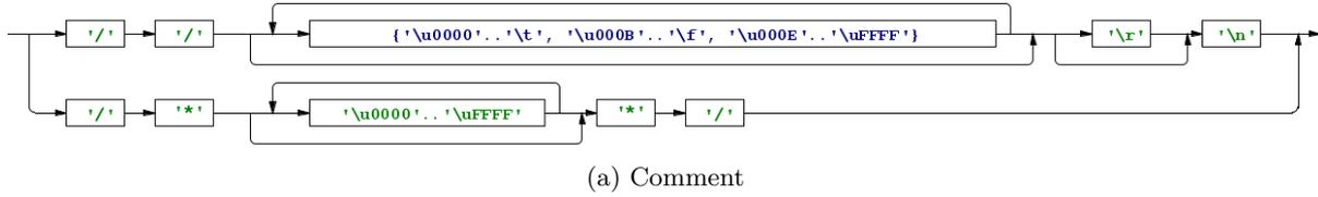
Figure B.5: Syntax diagrams representing the context-free grammar specified in the lexer source files for *comments*.
