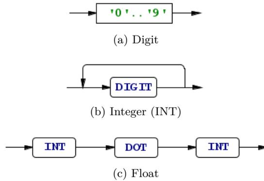
Figure B.1: Syntax diagrams representing the context-free grammar specified in the lexer source files for *numbers*.
