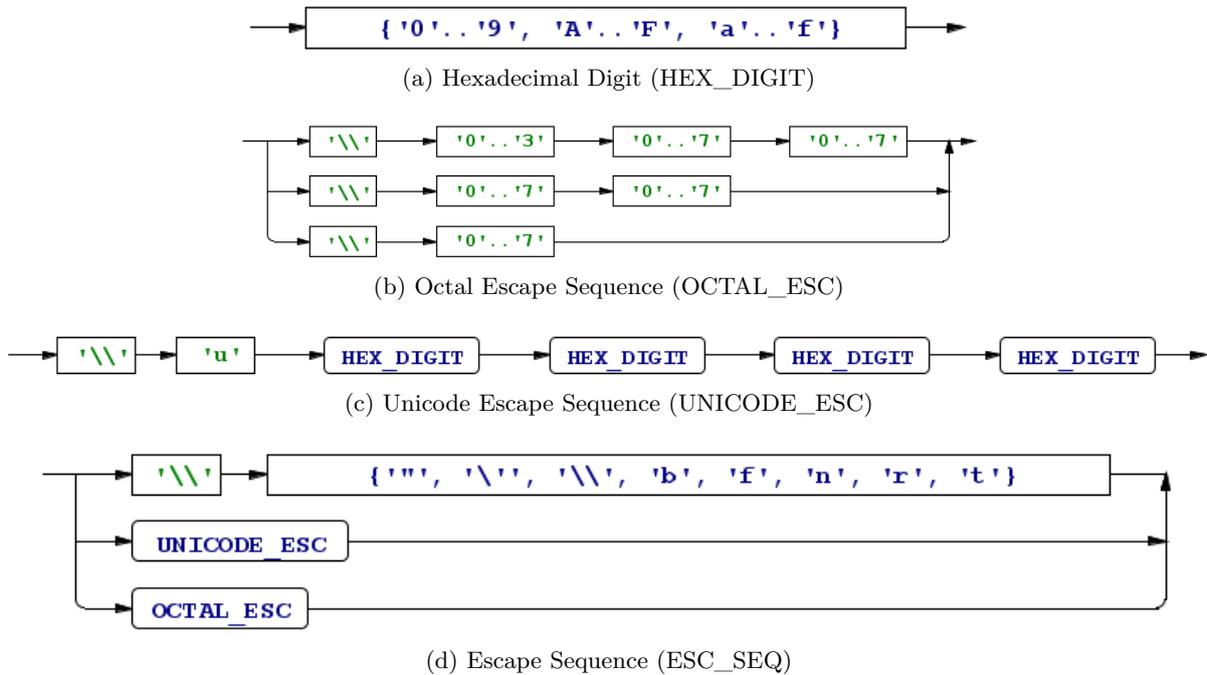
Figure B.4: Syntax diagrams representing the context-free grammar specified in the lexer source files for *escape sequences*.
