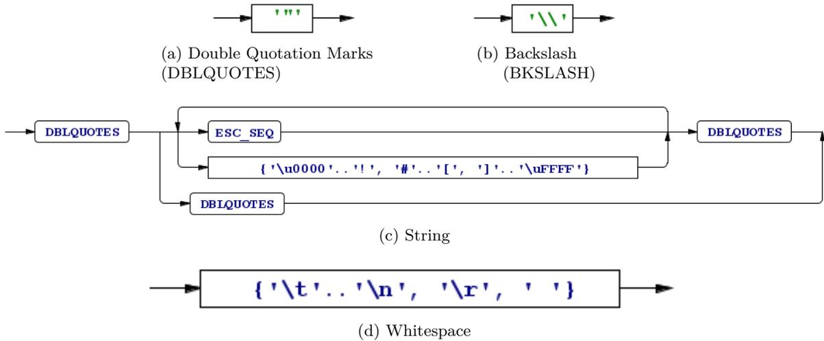
Figure B.3: Syntax diagrams representing the context-free grammar specified in the lexer source files for *strings* and *whitespace*.
