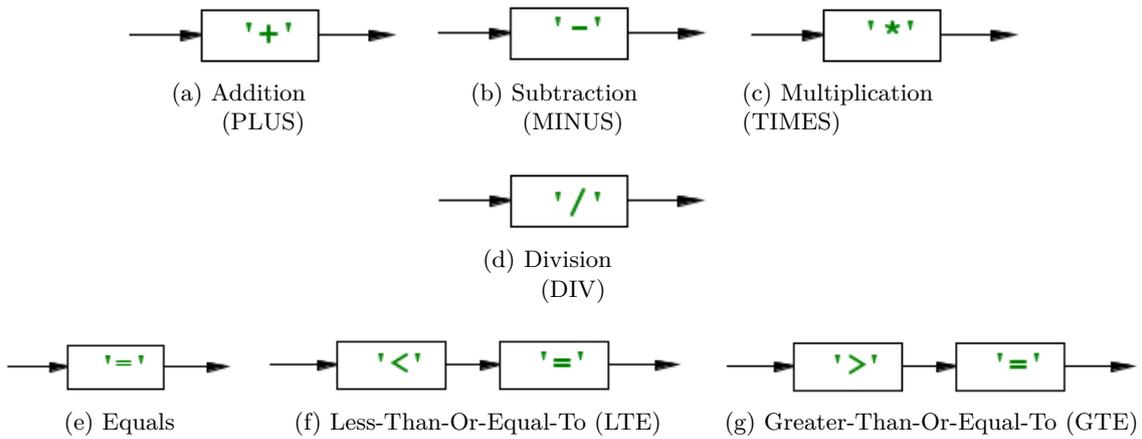
Figure B.6: Syntax diagrams representing the context-free grammar specified in the JADALexer source file for *mathematical operators*.
