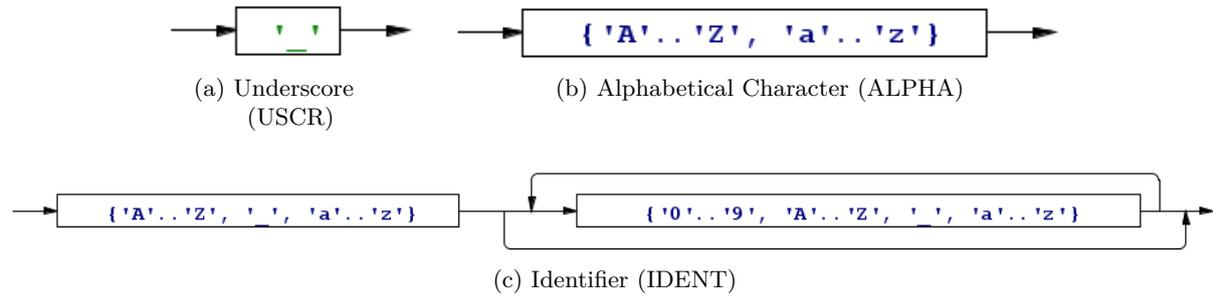
Figure B.2: Syntax diagrams representing the context-free grammar specified in the lexer source files for *variable identifiers*.
