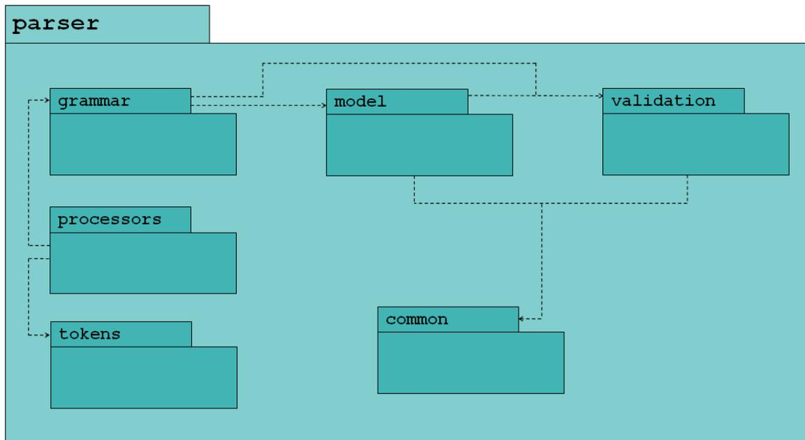
Figure 5.5: UML diagram showing the structure of the parser package, where the dashed arrows indicate the sub-package dependencies.
