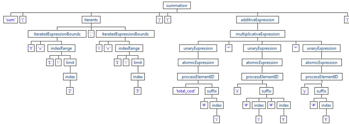
Figure 6.1: Diagram showing the interpretation of the *summation* parser rule for code listing 6.4 (line 4).
