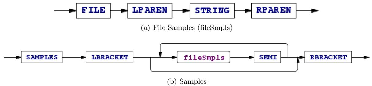
Figure B.13: Syntax diagrams representing the context-free grammar specified in the JADAParser source file for the *Samples* language construct.
