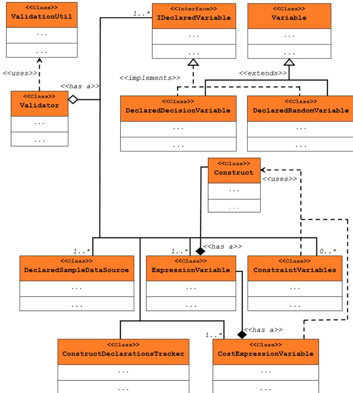
(b) UML class diagram illustrating the structural composition and dependencies of the Validator class.
