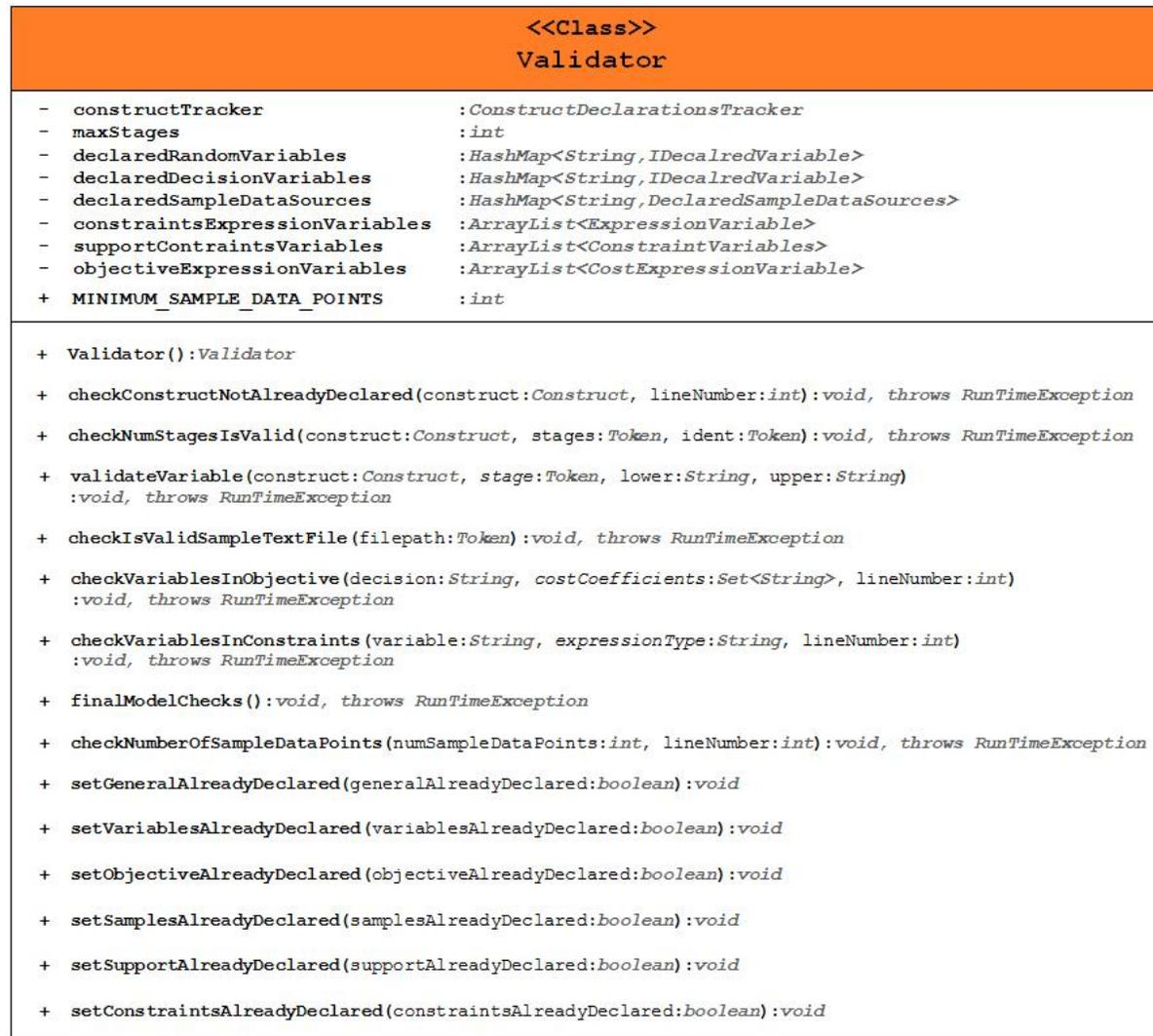
(c) UML class diagram explaining the functional behaviour of the Validator class.
