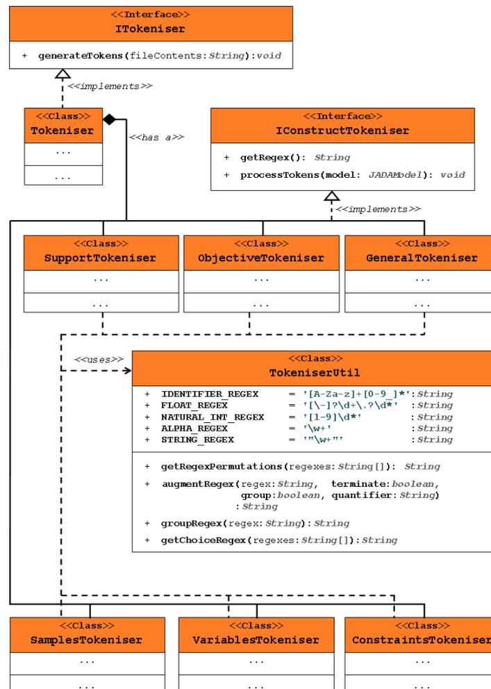
Figure 5.4: UML class diagram showing the structural implementation of the tokenisation component for the `Parser` class.
