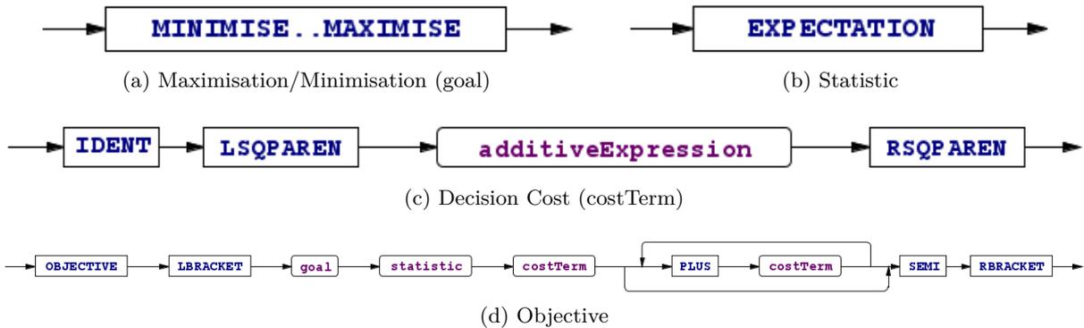
Figure B.14: Syntax diagrams representing the context-free grammar specified in the JADAParser source file for the *Objective* language construct.
