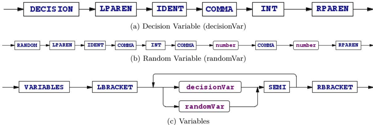
Figure B.10: Syntax diagrams representing the context-free grammar specified in the JADAParser source file for the *Variables* language construct.
