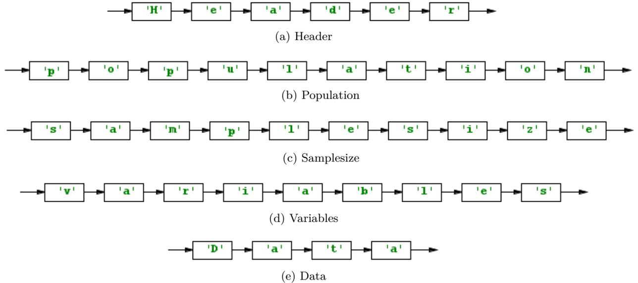
Figure B.8: Syntax diagrams representing the context-free grammar specified in the *SampleDataLexer* source file for the *reserved keywords*.
