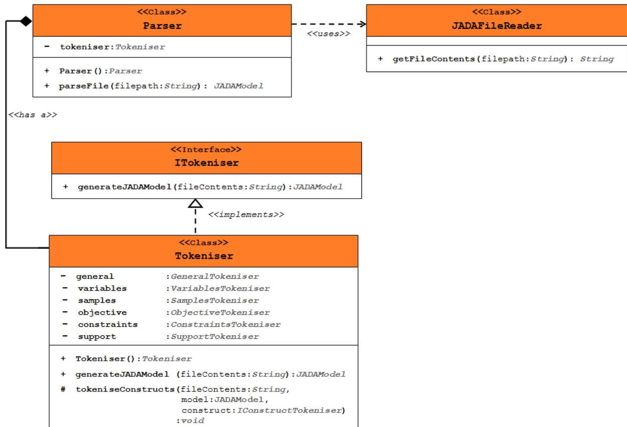
Figure 5.3: UML class diagram showing the structural implementation of the parser using MATLAB's regular expressions library.
