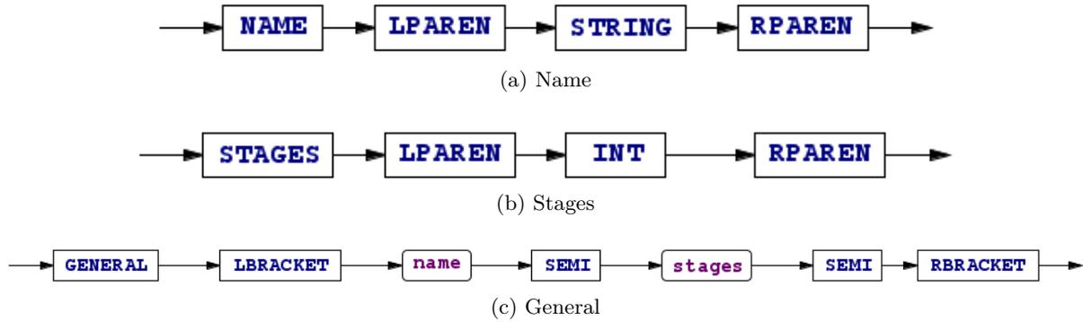
Figure B.9: Syntax diagrams representing the context-free grammar specified in the JADAParser source file for the *General* language construct.
