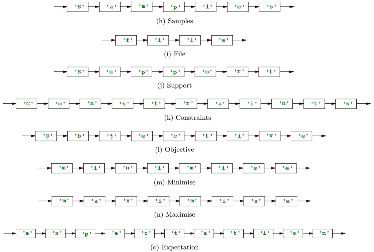
Figure B.8: Syntax diagrams representing the context-free grammar specified in the JADALexer source file for the *reserved keywords*.
