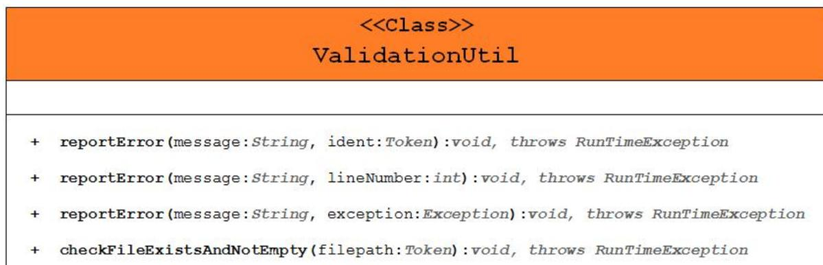
(a) UML class diagram specifying the utility functions provided by the `ValidationUtil` class.
