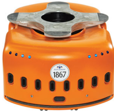
Figure 2.3: KIVA Systems' Autonomous Agent [13]
