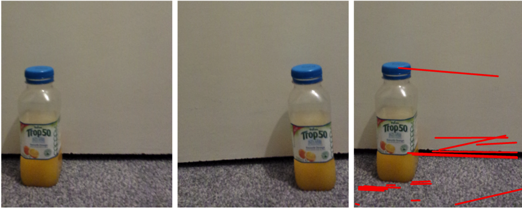
Figure 5.1: The first two images show the movement of the camera from left to right and the third image shows the feature displacement calculated by the optical flow
