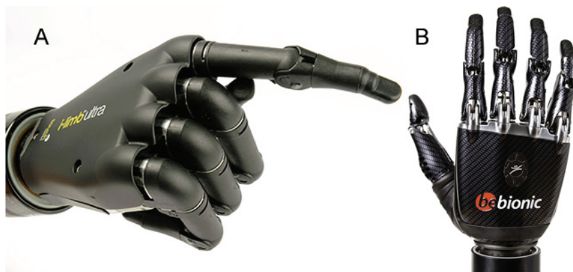
Figure 2.3: (A): i-limb ultra hand prosthesis (Touch Bionics). (B): bebionic3 prosthesis (RSLSteeper).
