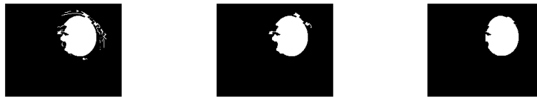
(d) Holes filled. (e) Remaining edges re-moved. (f) Mophological opening smooths edges.
