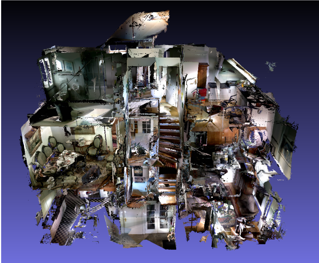
Figure 3.21: Front view of the the reconstructed house in full resolution. The final model consists of 44 million triangles with per-vertex colours. Backface culling was enabled to allow an unobstructed view into the rooms. Shading and lighting are disabled in the viewing program – real lighting is at work.
