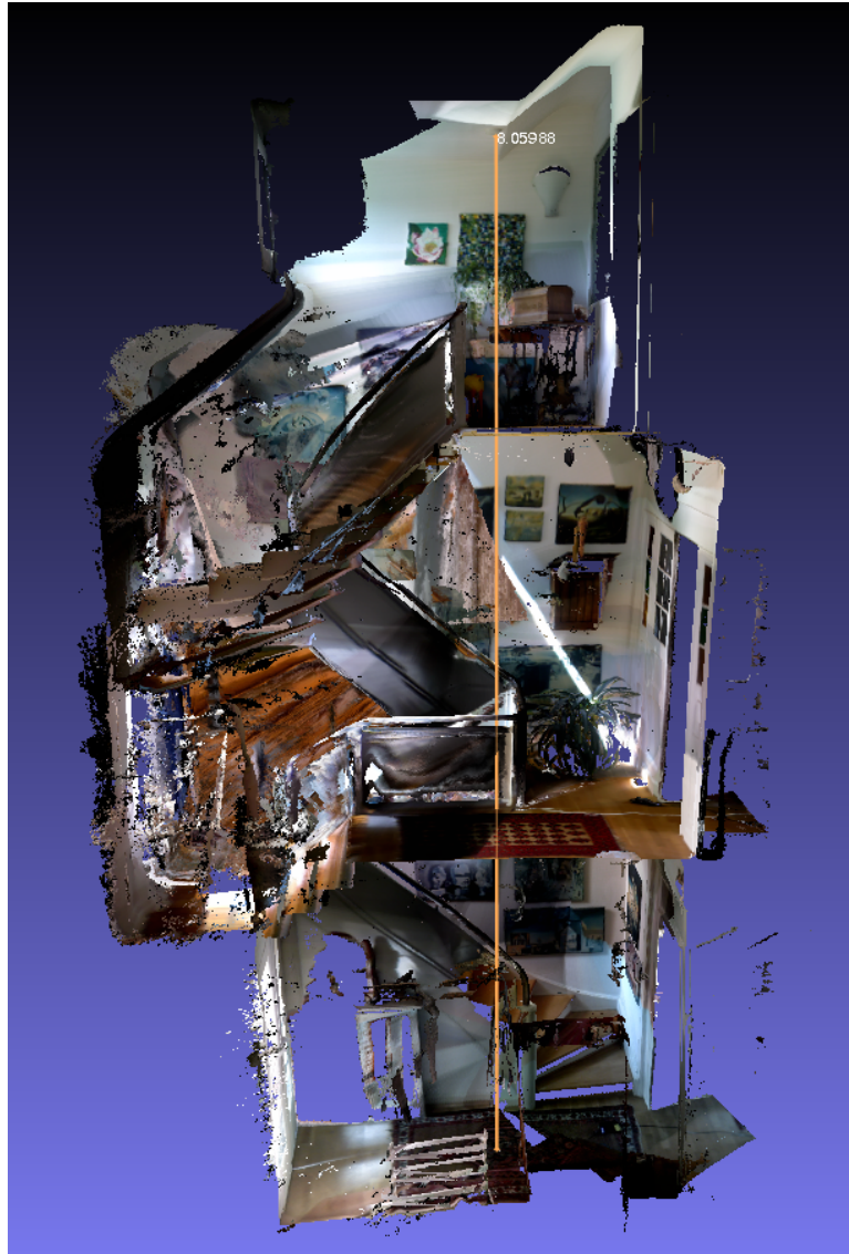
Figure 5.5: The height of the complete house is measured in the staircase across 3 levels.
