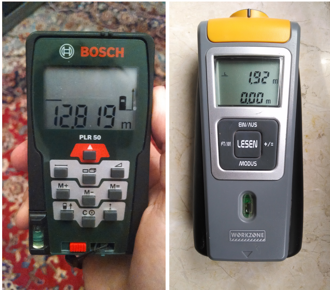
Figure 4.1: Left: A Bosch PLR 50 handheld laser rangefinder. Right: A WORKZONE commodity ultrasonic sensor.
