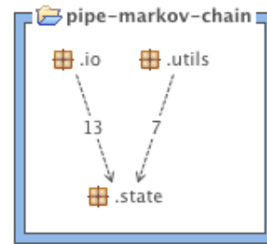
(e) The tangle graph for the new PIPEMarkovChain repository containing the classes which represent the underlying Markov chain of a Petri net and the explored sets data structure. It reports 0 tangles.
