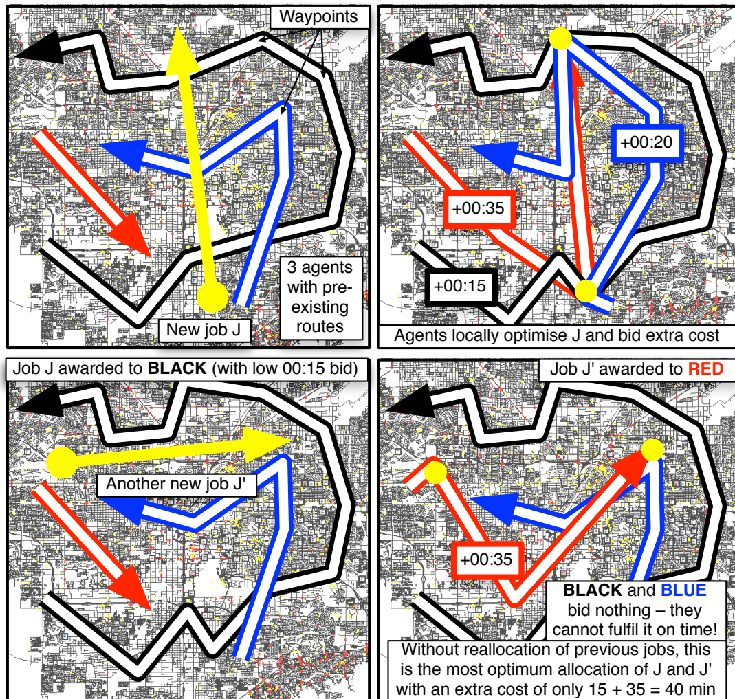
FIGURE 7.4: An example of CNP optimally allocating two jobs, J and J' , that arrive in sequence. The figure is to be read left-to-right, top-down.
