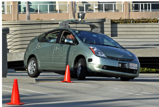
FIGURE 2.2: A Toyota Prius modified by Google to operate as a driverless car [12].
