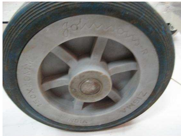
Figure 5.7: Johnson 150x40 wheel used on the robot.
