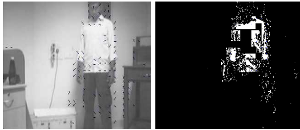
Figure 4.7: Robot is able to track the person when the background color is same. Since we look for patches which have discontinuity in motion and intensity as well, the background patches having similar color may tend to be ruled out due to their uniform intensity profile and continuity in motion as the flow vectors are smoothly aligned after the energy minimization process.
