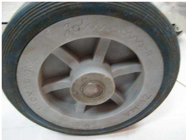
Figure 2.6: Johnson 150x40 wheel used on the robot.
