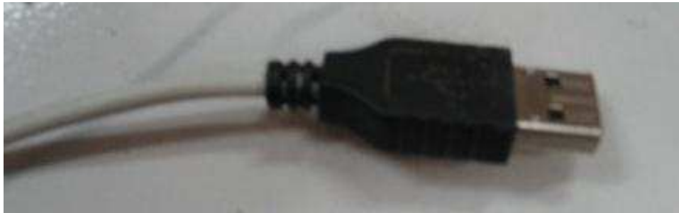
Figure 2.4: The figure shows USB cable and plug A at the end.
