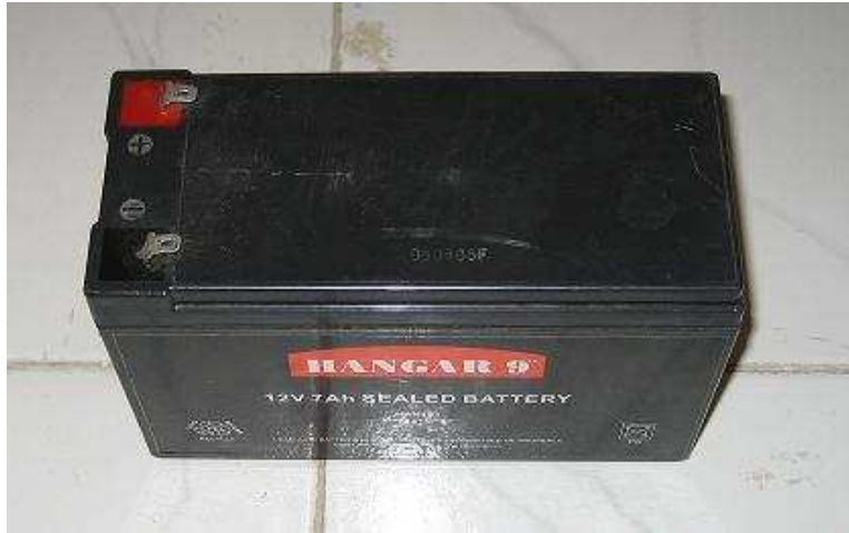
Figure 2.3: A typical 12V, 7Ah Lead Acid battery.
