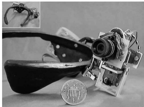
**Figure 2. Collar-mounted wearable robot equipped with a miniature camera manipulated by a three-axis motorized active platform.**
