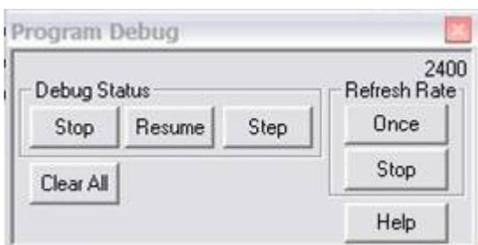
This is the main debugger window for controlling user program execution. The buttons on this window allow you to start/stopm suspend/resume and program execution. Other buttons allow you to control the rate at which information from your robot is refreshed.
