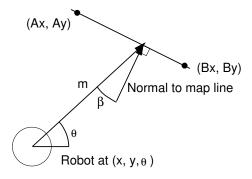
Possibly relevant for real sensors may be the angle between the sonar direction and the normal to the wall. If this is too great, probably the sonar will not give a sensible reading and you should ignore it.
