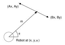
• If robot is at pose  $(x, y, \theta)$  then its forward distance to an infinite wall passing through  $(A_x, A_y)$  and  $(B_x, B_y)$  is:
