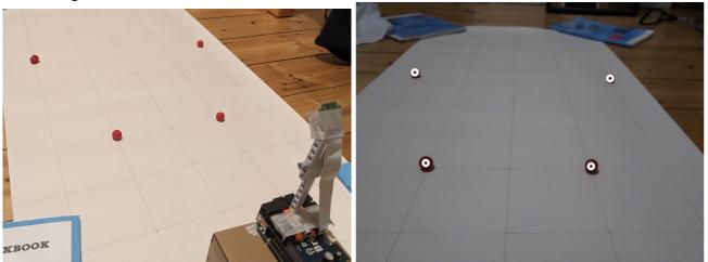
We have provided a program which will detect the positions of markers in the image from the camera, and display and print out the image coordinates.
