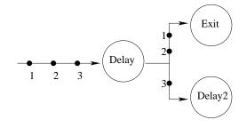
which routes class 1 and 2 customers to the exit node and class 3 customers to the internal node.
