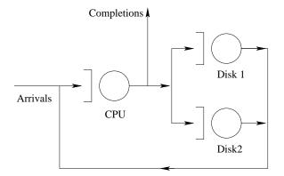
Jobs arrive according to a Poisson process and join the CPU. The mean CPU visit time is 5ms. At the end of a visit the job either leaves (probability 1 in 121 visits) or visits one of two disks (probabilities 70/121 and 50/121 respectively). The disk service times are 30ms and 27ms respectively. All time delays are exponential. The code here shows one run of the model over 10000 completed jobs.
