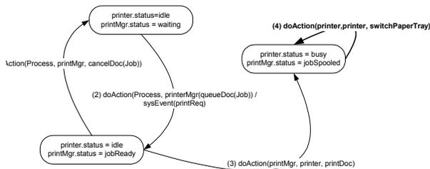
Figure 4: State chart for Printer system functionality.
