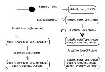
Figure 5: UML state chart for DiffServRouter type
