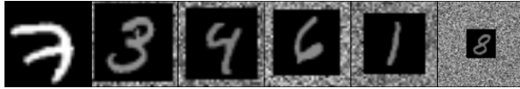
Figure 2: Sample images of MNIST digits embedded into background images with percentage of uninformative noise of 0%, 18.4%, 32.2%, 42.7%, 51% and 88.9% from left to right.
